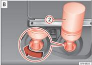
Fig. 237 AdBlue tank with filler neck cap and refilling bottle
