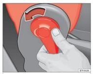
**Fig. 160** Unlocking the folding backrest of the front passenger seat
