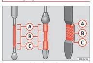
Fig. 241 Marked engine oil dipstick
