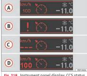
Fig. 218 Instrument panel display: CCS status indications
