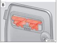
**Fig. 165** Remove the shelf supports A then put them away safely B.
