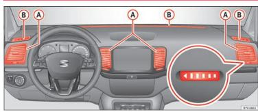
Fig. 196 Air vents in the dash panel
