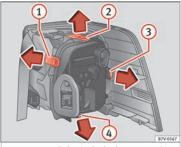
Fig. 114 Rear lights in the body: Remove the bulb holder. 1 to 4: Attachment tab
