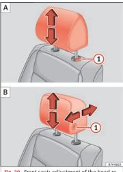
**Fig. 20** Front seat: adjustment of the head restraint.
