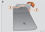
Fig. 167 Third seat row: fold down the rear seat to load A then return to position B
