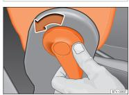
Fig. 164 Unlocking the folding backrest of the front passenger seat
