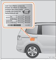
Fig. 301 Position of tyre pressure specification plate
