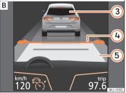
Fig. 262 On the instrument panel display: (A) ACC inactive (Standbu), (B) ACC active.
