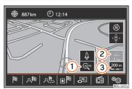
**Fig. 229** Messages and function buttons on the map display.
