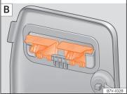
Fig. 169 Remove the shelf supports A then put them away safely B.
