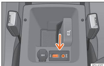
Fig. 231 Centre front armrest: USB/AUX-IN input.
