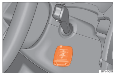
Fig. 235 Emergency ignition in vehicles with Keyless Access.
