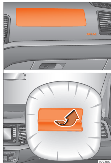
Fig. 17 Front passenger airbag located in dash panel.
