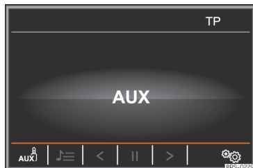
Fig. 210 Media Mode: external audio source connected to the AUX-IN socket.
