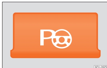
Fig. 269 Detailed view of the centre console: button to switch the park assist system on manually. »
