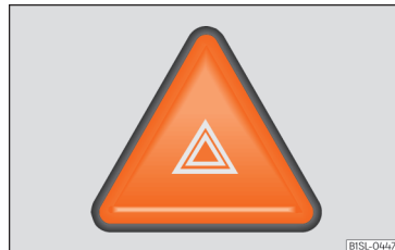
Fig. 117 Dash panel: hazard warning lights switch
