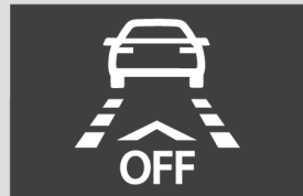
Fig. 253 On the instrument panel display: Front Assist deactivated indication.
