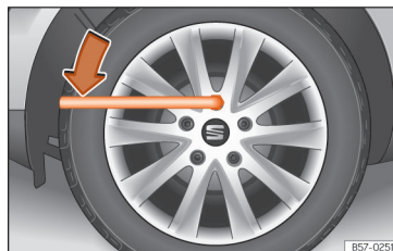
Fig. 45 Wheel change: loosen the wheel nuts.
