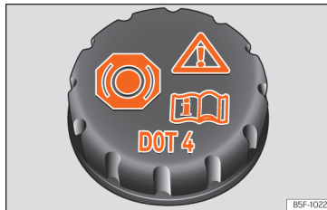
Fig. 292 Engine compartment: brake fluid reservoir cap.
