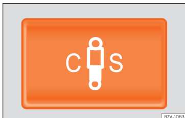
Fig. 243 In the centre console: button to adjust the adaptive suspension.
