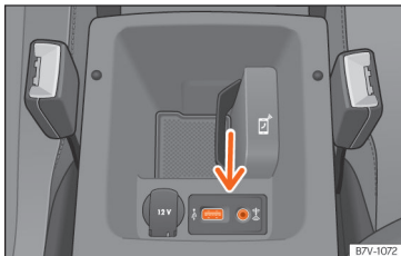
Fig. 185 Centre front armrest: USB/AUX-IN input.
