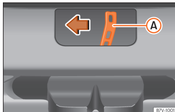
Fig. 108 Detail of the luggage compartment: emergency unlocking
