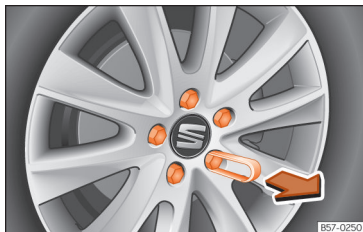
Fig. 43 Wheel: wheel nuts with caps.
