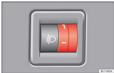
Fig. 148 Dash panel: headlight range control.
