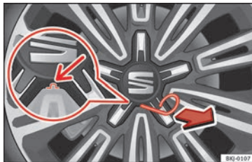
Fig. 78 Removing the central wheel trim.
