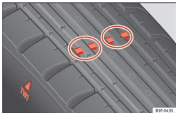
Fig. 240 Tyre tread wear indicators.
