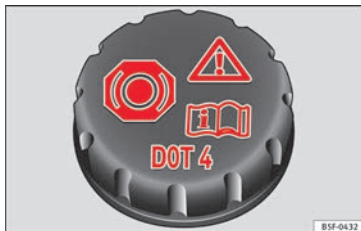
Fig. 68 Engine compartment: brake fluid reservoir cap.
