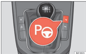
Fig. 209 In the centre console: button to switch on the Park Assist system.
