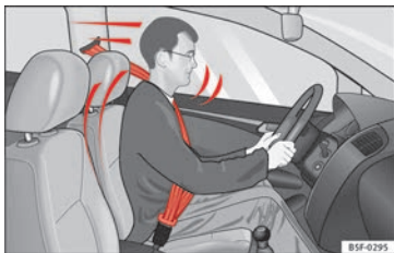
Fig. 98 Drivers with properly worn seat belts will not be thrown forward in the event of sudden braking.
