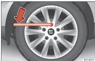
Fig. 81 Changing a wheel: loosen the wheel bolts.
