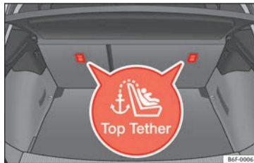
Fig. 32 Position of the Top Tether rings on the back of the rear seat.
