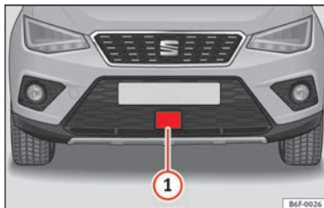
Fig. 190 On the front bumper: radar sensor.
