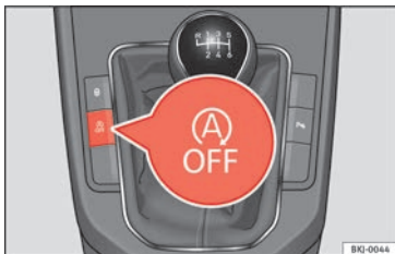
Fig. 184 Centre console: Start-Stop system button.
