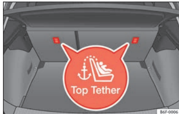
Fig. 36 Position of the Top Tether rings on the back of the rear seat.
