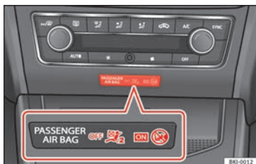
Fig. 23 Centre side of dash panel: control lamp for deactivated front passenger airbag in centre console.
