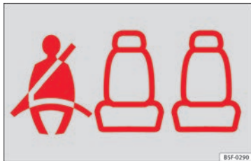
Fig. 97 Instrument panel: right rear seat occupied and corresponding seat belt fastened display.
