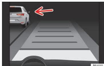
Fig. 198 On the instrument panel display: ACC active, vehicle detected in an outer lane.
