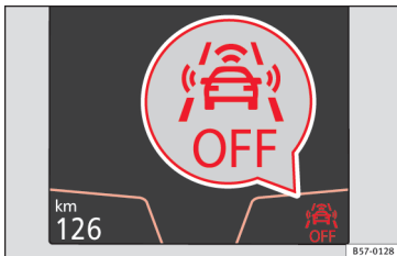
Fig. 191 On the instrument panel display: Front Assist switched off message.
