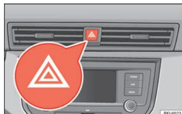
Fig. 41 Dash panel: switch for hazard warning lights.
