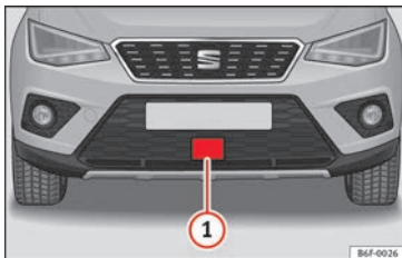
Fig. 195 On the front bumper: radar sensor.
