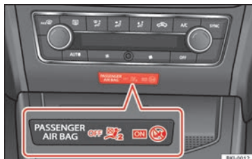
Fig. 104 Centre side of dash panel: control lamp for deactivated front passenger airbag in centre console.
