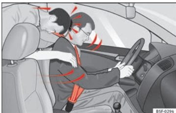
Fig. 100 The unbelted passenger in the rear seat is thrown forward violently, hitting the driver who is wearing a seat belt.
