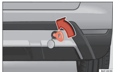
Fig. 86 Right side of the rear bumper: Towing ring.
