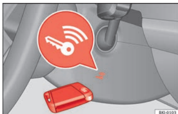
Fig. 177 On the right of the steering column: emergency start.
