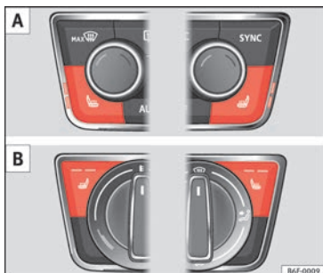
Fig. 154 In the centre console: front seats heating switch A : version with Climatronic. B : version with manual air conditioning.
