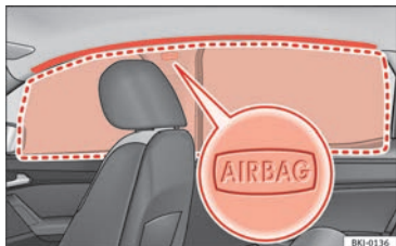
Fig. 26 Location and deployment area of the head-protection airbag.
