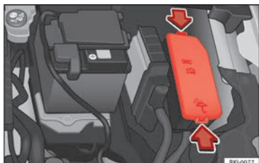
Fig. 71 In the engine compartment: fuse box cover.
