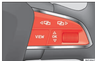
Fig. 47 Right side of multifunction steering wheel: control buttons.
