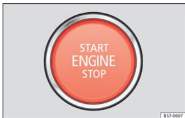
Fig. 176 In the lower part of the centre console: starter button.
