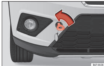
Fig. 85 Right side of the front bumper: Towing ring.
