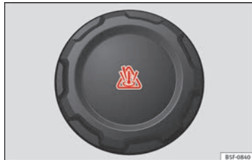
Fig. 67 Engine compartment: coolant expansion tank cap.
