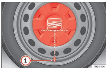
Fig. 77 Correct positioning of the central wheel trim for steel rims.
