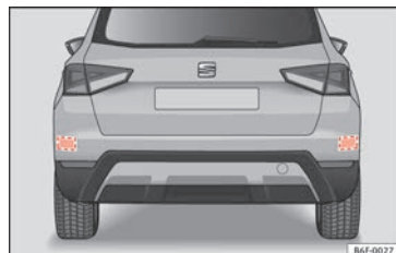
Fig. 202 Rear view of the vehicle: radar sensor zones.
