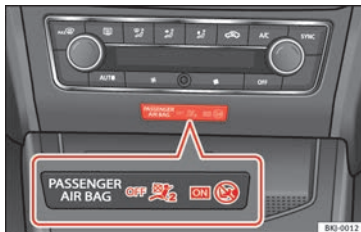
Fig. 56 Warning lamp for disabling the front passenger airbag.
