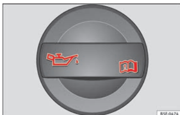
Fig. 66 In the engine compartment: Engine oil filler cap.
