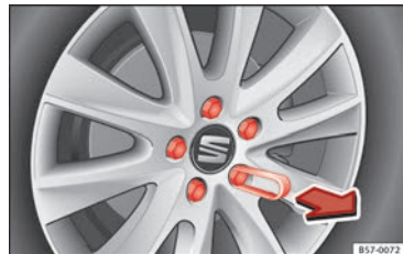
Fig. 80 Wheel: wheel bolts with caps.
