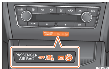
Fig. 95 Centre of the instrument panel: control lamp for deactivated front passenger airbag in centre console.
