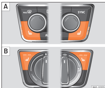
Fig. 150 On the centre console: front seats heating switch [A]: version with Climatronic, [B]: version with manual air conditioning.
