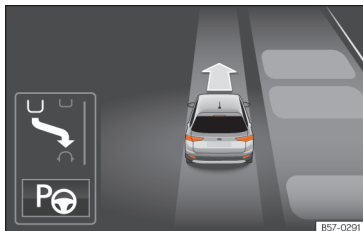
Fig. 250 On the instrument panel display: display of the assisted parking system with decreased visibility.
