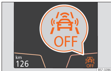
Fig. 232 On the screen of the instrument panel Front Assist switched off message.
