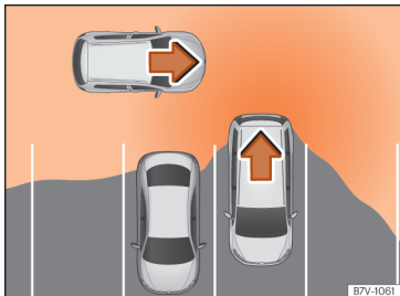
Fig. 246 Diagram of the parking assistant: detected area around the vehicle that is driving off.
