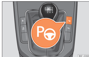
Fig. 248 In the centre console: button to switch on the Park Assist system.
