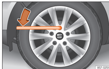
Fig. 72 Tyre change: slacken the wheel bolts.
