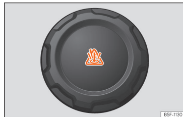
Fig. 60 Engine compartment: coolant expansion tank cap.
