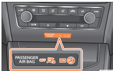
Fig. 25 Centre of the instrument panel: control lamp for deactivated front passenger airbag in centre console.
