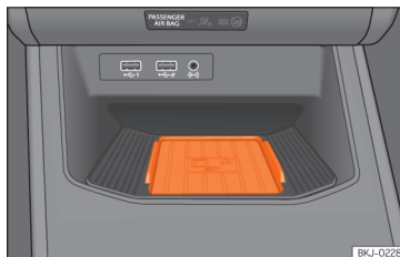
Fig. 207 In the centre console: pad for the mobile phone connection.
