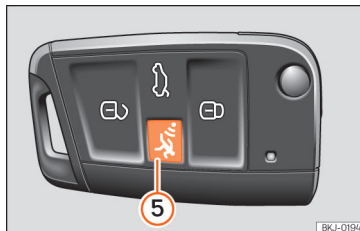
Fig. 87 Vehicle key with alarm button.
