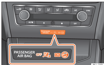
Fig. 18 Central part of the dashboard: control lamp for the deactivation of the front passenger front airbag.
