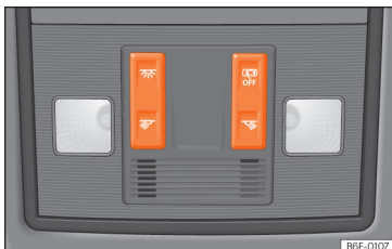
Fig. 111 Detail of roof lining: front lighting of the passenger compartment.
