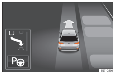
Fig. 248 On the instrument panel display: view of the parking assist system with reduced view.
