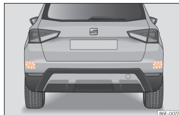
Fig. 241 Rear view of the vehicle: radar sensor zones.
