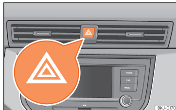
Fig. 108 Dash panel: hazard warning lights switch
