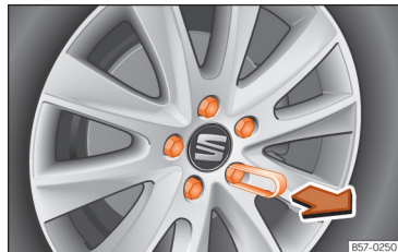
Fig. 35 Wheel: wheel nuts with caps.
