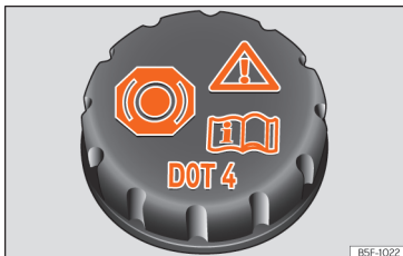
Fig. 286 Engine compartment: brake fluid reservoir cap.
