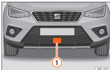
Fig. 228 On the front bumper: radar sensors.
