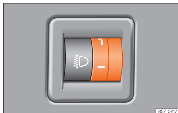
Fig. 109 Next to the steering wheel: headlight range control.
