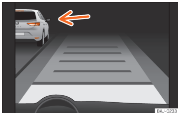
Fig. 237 On the instrument panel display: ACC active, vehicle detected in an outer lane.
