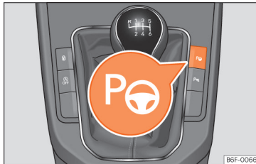
Fig. 247 In the centre console: button to switch on the Park Assist system.
