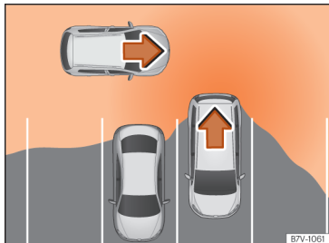
Fig. 167 Schematic representation of the rear cross traffic alert assistant: zone monitored around the vehicle while leaving a parking space.
