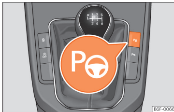
Fig. 169 In the centre console: button to switch on the Park Assist system.
