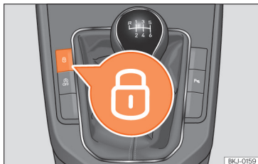
Fig. 82 Centre console: central locking button.
