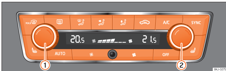
Fig. 119 In the centre console: Climatronic controls.
