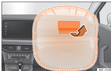
Fig. 15 Front passenger airbag located in dash panel.
