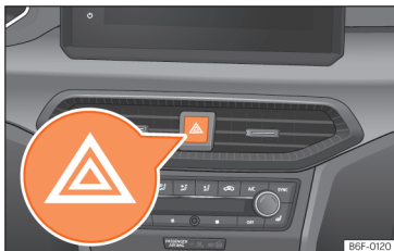
Fig. 95 Dash panel: hazard warning lights switch
