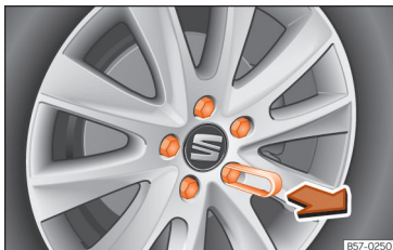
Fig. 33 Wheel: wheel nuts with caps.
