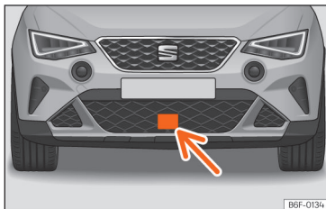
Fig. 139 On the front bumper: radar sensors.
