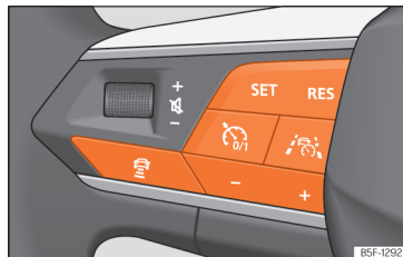
Fig. 157 Left side of the multifunction steering wheel: buttons for operating Travel Assist.
