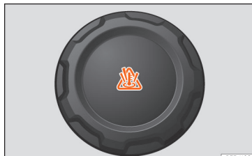
Fig. 197 Engine compartment: coolant expansion tank cap.
