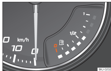
Fig. 65 Analogue instrument panel: fuel gauge
