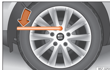
Fig. 35 Wheel change: loosen the wheel nuts.
