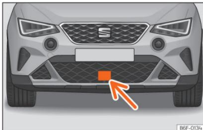
**Fig. 139** On the front bumper: radar sensors.
