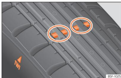
Fig. 203 Tyre profile: tread wear indicators.
