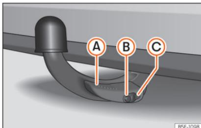
**Fig. 181** Tow hook fixed correctly
