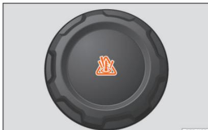
**Fig. 198** Engine compartment: coolant expansion tank cap.
