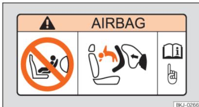
**Fig. 22** Airbag sticker: on the passenger's sun visor
