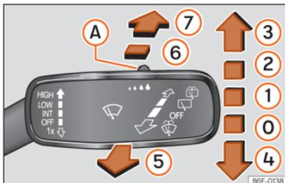
**Fig. 98** Operating the windscreen wiper and rear wiper.
