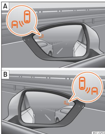
**Fig. 158** Control lamp of the lane departure warning.
