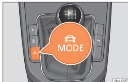
**Fig. 138** Next to the gear lever: MODE button.
