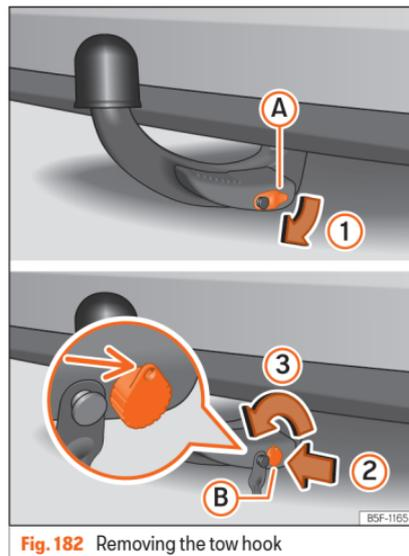
**Fig. 182** Removing the tow hook
