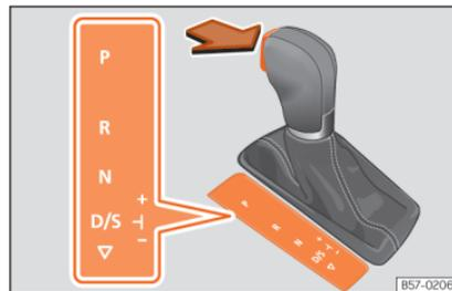
Fig.134 Selector lever lock.
