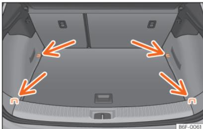
**Fig. 112** Location of fastening rings in luggage compartment.
