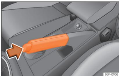
**Fig. 162** Handbrake between the front seats.
