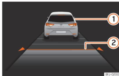
**Fig. 150** On the instrument panel display: ACC active.
