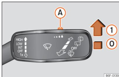
Fig. 99 Wiper lever: adjust the rain sensor (A)
