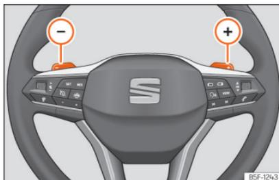
Fig. 136 Steering wheel: automatic transmission levers
