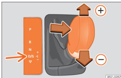
Fig. 135 Lever in the Tiptronic position
