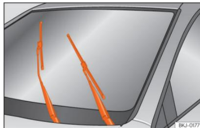
**Fig. 39** Wipers in service position.
