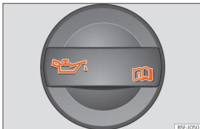
**Fig. 196** In the engine compartment: Engine oil filler cap.
