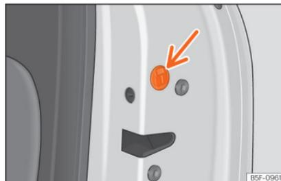
**Fig. 87** Locking the door manually.
