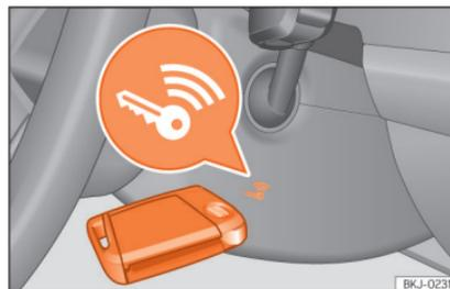
**Fig. 131** On the right of the steering column: emergency start.
