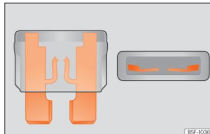
**Fig. 50** Image of a blown fuse.
