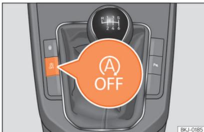
**Fig. 132** Centre console: Start-stop system button.
