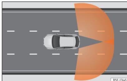
**Fig. 143** Sensor detection zones
