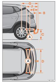
Fig. 185 Limits and attachment points for retrofitting a towing bracket.
