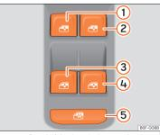
Fig. 91 Detail of the driver's door: window controls.
