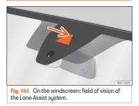
Depending on the equipment, the vehicle may be fitted with a front camera on the front windscreen **»** Fig. 141. This camera detects lane boundaries (lines) to provide support for the following functions:
