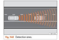
A radar sensor may be fitted to the front bumper of the vehicle **>>> Fig. 139**. The front radar detects any objects in its detection zone **>>> Fig. 140** and provides support for the following functions:
