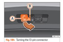
• Grip the connector in area (A) and remove it in the direction of the arrow **>>>** Fig. 184.
