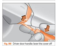
If the central locking system should fail to operate, the driver door can still be locked and unlocked by turning the key in the lock. As a general rule, when the driver door is locked manually all other doors are locked. When it is unlocked manually, only the driver door opens. Please observe the instructions relating to the anti-theft alarm system **»** page 103.
