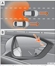
Fig. 160 Schematic representation: A Situation of passing and then moving into the righthand lane. B Indication from the blind spot detector in the right-hand external mirror.
