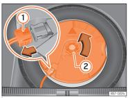
**Fig. 205** In the luggage compartment: remove the subwoofer.
