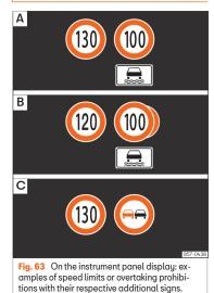
The traffic sign detection system records the standard traffic signs in front of the vehicle with a camera located on the base of the interior mirror and provides information about speed limits and overtaking prohibitions.
