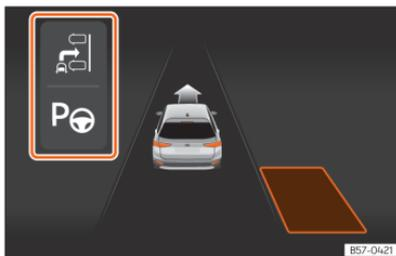
**Fig. 124** On the instrument panel display: display of the assisted parking system with decreased visibility.
