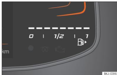
Fig. 5 Basic instrument cluster: fuel gauge.
