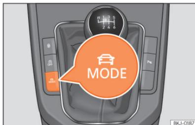
**Fig. 92** Next to the gearbox lever: MODE button.
