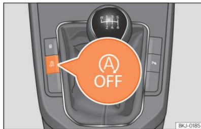
**Fig. 86** Centre console: Start-Stop system button.
