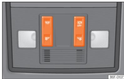
**Fig. 74** Detail of headliner: front interior lighting.
