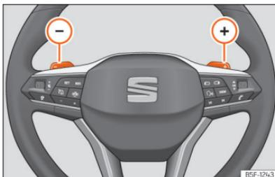
**Fig. 90** Steering wheel: automatic gearbox levers
