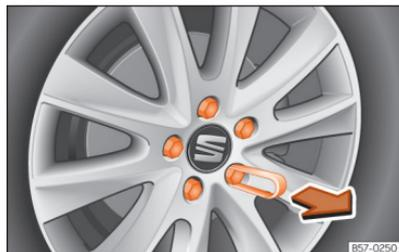
**Fig. 194** Wheel: wheel bolts with caps.
