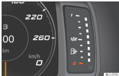
Fig. 6 SEAT Digital Cockpit instrument cluster: fuel gauge.
