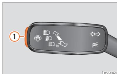
**Fig. 93** On the turn light and main beam lever: key for driver assistance systems (depending on the version).
