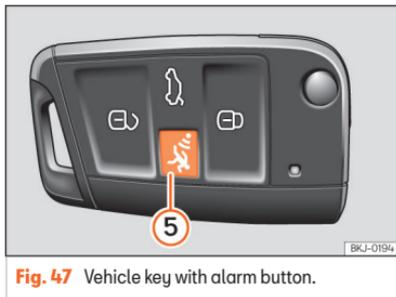
Fig. 47 Vehicle key with alarm button.
