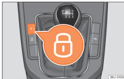
**Fig. 53** Centre console: central locking switch.
