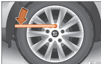
**Fig. 196** Tyre change: slacken the wheel bolts.
