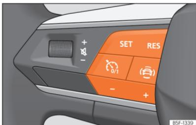
**Fig. 101** On the multifunction steering wheel: cruise control operation buttons.
