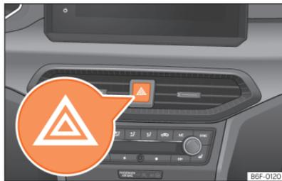
**Fig. 44** Dashboard: switch for hazard warning lights.
