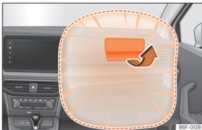
**Fig. 29** Front passenger airbag located in dash panel.
