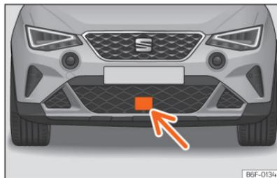
**Fig. 95** On the front bumper: radar sensor.
