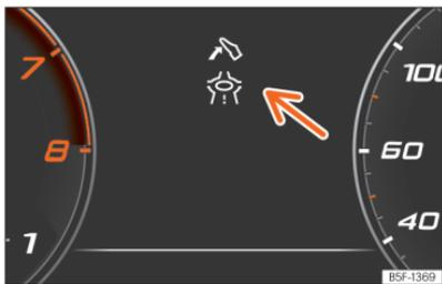
**Fig. 12** Eco-efficient driving assistance indication (schematic representation).
