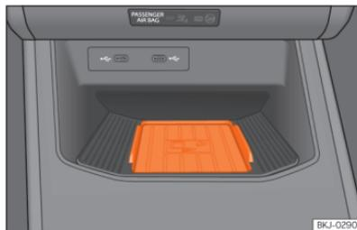
**Fig. 142** Centre console: slot for mobile phone connection.
