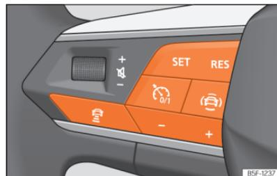
**Fig. 104** On the multifunction steering wheel: buttons for operating the ACC.
