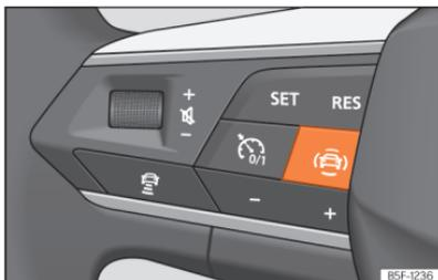
**Fig. 94** Left side of the multifunction steering wheel: button for driver assistance systems [depending on the version].
