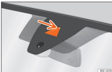
**Fig. 97** On the windscreen: field of vision of the Lane Assist system camera.
