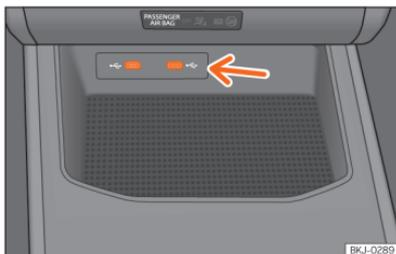
**Fig. 135** Centre console: USB input.
