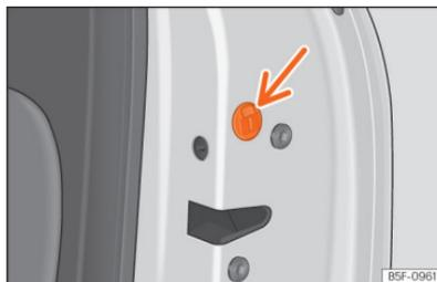
**Fig. 56** Locking the door manually.
