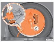
Fig. 192 In the boot: remove the subwoofer.
