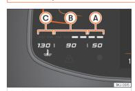
**Fig. 8** Basic digital instrument cluster: engine coolant temperature display.
