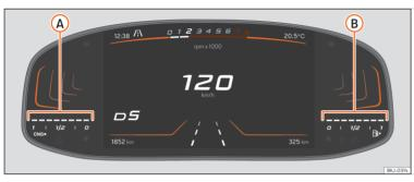
Fig. 7 Instrument cluster: natural gas gauge
