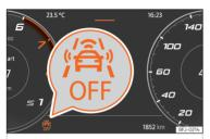
**Fig. 110** On the screen of the instrument panel Front Assist switched off message.
