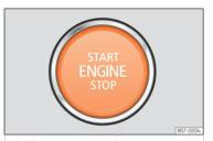
**Fig. 84** In the lower part of the centre console: start button.
