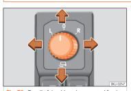
Fig. 79 Detail of the driver door; control for the exterior mirror
