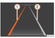
**Fig. 111** On the instrument cluster screen: indications of the lane assist system.
