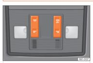
Fig. 74 Detail of headliner: front interior lighting.
