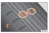
Fig. 190 Tyre profile: tread wear indicators.
