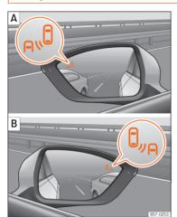
**Fig. 114** Control lamp of the lane departure warning.
