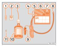
**Fig. 201** Standard display: contents of the anti-puncture kit.
