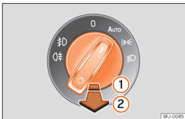
Fig. 71 Instrument panel: light panel.
