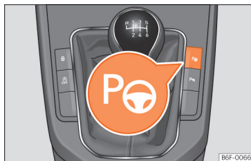
Fig. 122 In the centre console: button to switch on the Park Assist system.
