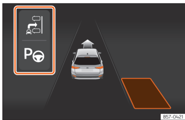
Fig. 123 On the instrument panel display: display of the assisted parking system with decreased visibility.
