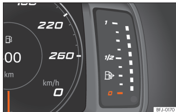
Fig. 6 SEAT Digital Cockpit instrument cluster: fuel gauge.
