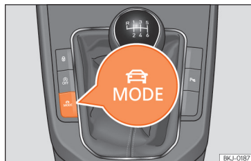
Fig. 91 Next to the gearbox lever: MODE button.
