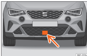
Fig. 94 On the front bumper: radar sensor.
