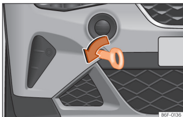
Fig. 163 Right side of the front bumper: towline anchorage screwed in.
