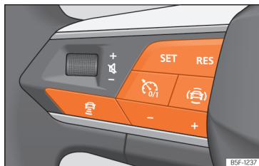
Fig. 103 On the multifunction steering wheel: buttons for operating the ACC.
