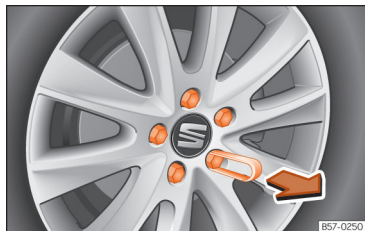
Fig. 192 Wheel: wheel bolts with caps.
