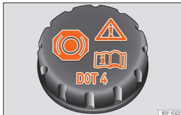
Fig. 180 Engine compartment: brake fluid reservoir cap.
