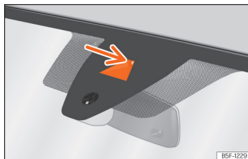
Fig. 96 On the windscreen: field of vision of the Lane Assist system camera.
