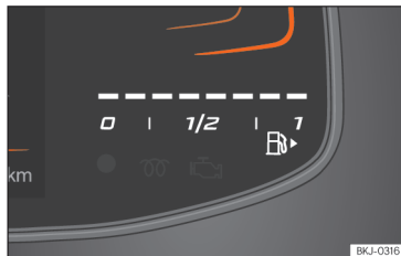
Fig. 5 Basic instrument cluster: fuel gauge.
