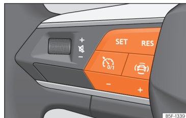
Fig. 101 On the multifunction steering wheel: buttons to control the speed limiter.
