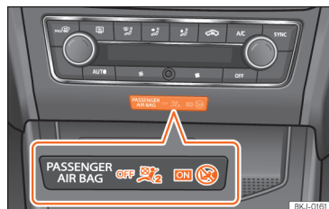
Fig. 30 Centre of the instrument panel: control lamp for deactivated front passenger airbag in centre console.
