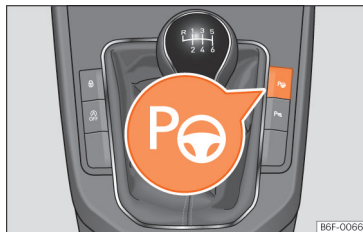
Fig. 125 In the centre console: button to switch on the Park Assist system.
