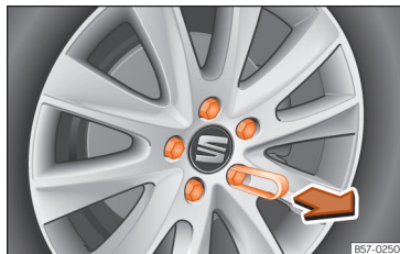
Fig. 195 Wheel: wheel bolts with caps.
