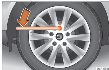
Fig. 197 Tyre change: slacken the wheel bolts.
