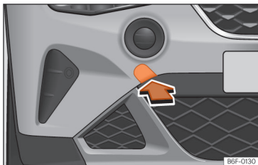
Fig. 165 Front bumper on right: remove the lid.
