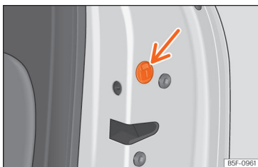
Fig. 55 Locking the door manually.
