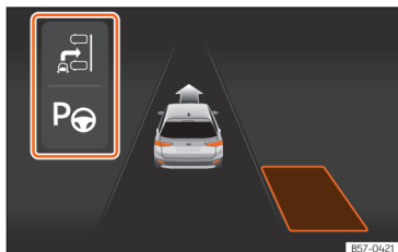
Fig. 126 On the instrument panel display: display of the assisted parking system with decreased visibility.
