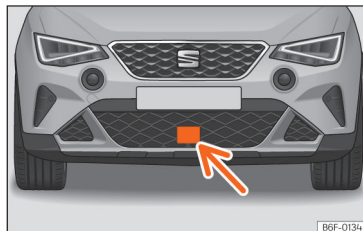
Fig. 94 On the front bumper: radar sensor.
