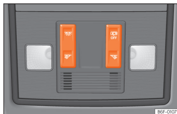
Fig. 73 Detail of headliner: front interior lighting.
