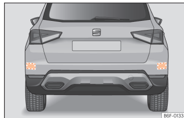
Fig. 97 Rear view of the vehicle: radar sensor areas.
