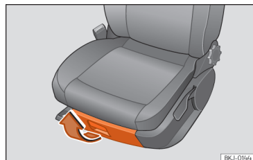
Fig. 135 Storage compartment under the right front passenger seat.
