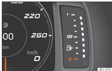
Fig. 6 SEAT Digital Cockpit instrument cluster: fuel gauge.
