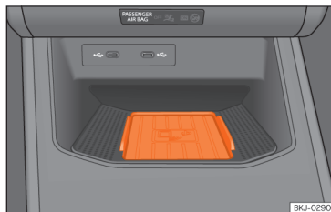
Fig. 144 On the centre console: pad for the mobile phone connection.
