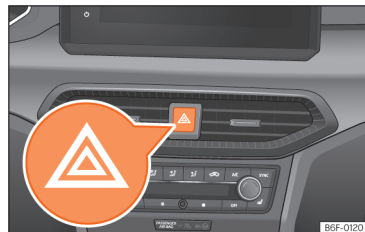
Fig. 43 Dashboard: switch for hazard warning lights.
