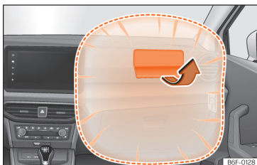
Fig. 28 Front passenger airbag located in dash panel.
