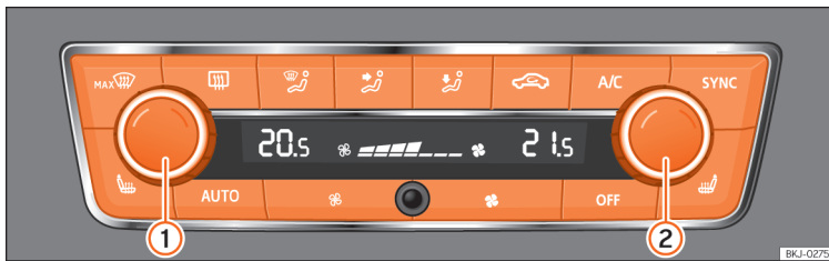
Fig. 80 In the centre console: Climatronic control panel.
