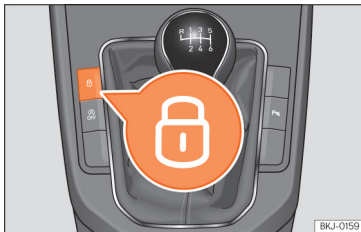
Fig. 52 Centre console: central locking switch.
