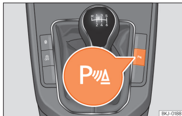
Fig. 122 Centre console: parking aid button (depending on the version).
