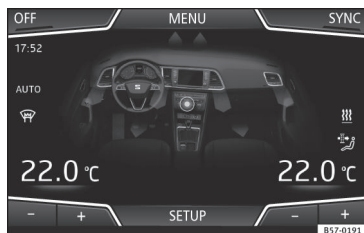
Afb. 155 Scherm van Easy Connect: menu Airconditioning.
