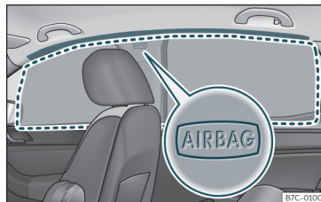
Fig. 20 Location of head-protection airbags.
