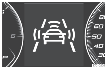
Fig. 210 On the instrument panel display: advance warning indications.
