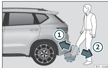
Fig. 80 Rear lid with sensor-controlled opening (Easy Open).
