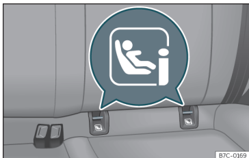
Fig. 24 Rear seat: ISOFIX/i-Size securing rings.
