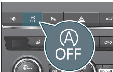
Fig. 199 Centre console: Start-stop system button.
