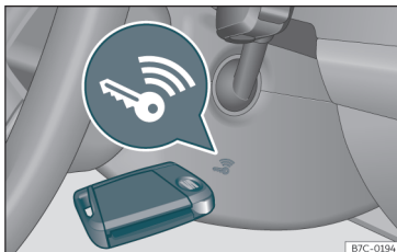
Fig. 198 On the right of the steering column: emergency start.
