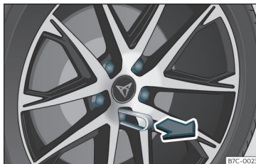
Fig. 30 Wheel: wheel nuts with caps.
