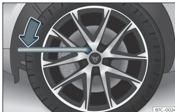
Fig. 32 Wheel change: loosen the wheel nuts.
