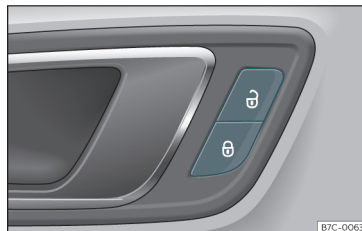
Fig. 70 Driver's door: central locking switch.
