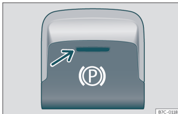
Fig. 230 In the lower part of the centre console: electronic parking brake button
