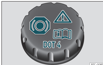
Fig. 261 Engine compartment: brake fluid reservoir cap.
