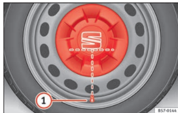
Fig. 69 Correct position of the central wheel trim for steel wheels.
