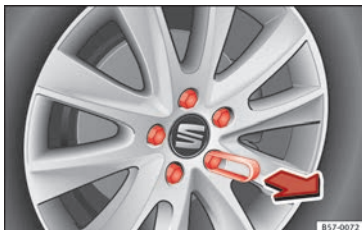
Fig. 70 Wheel: wheel bolts with caps.
