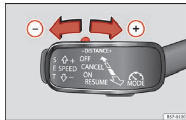
Fig. 183 Control lever: setting the distance.
