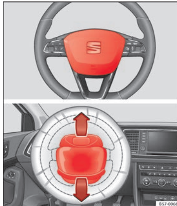
Fig. 20 Driver airbag located in steering wheel.
