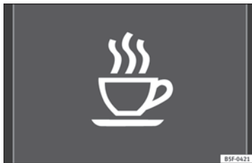
Fig. 201 On the instrument panel display: fatigue detection symbol.
