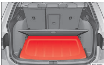
Fig. 153 In the luggage compartment: fitting the storage compartment shelf.
