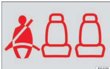
Fig. 87 Instrument panel: right rear seat occupied and corresponding seat belt fastened display.
