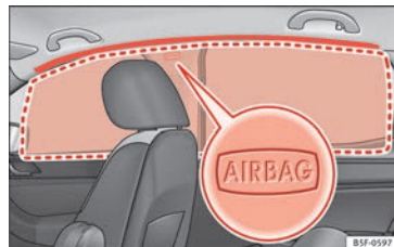
Fig. 27 Location of head-protection airbags.
