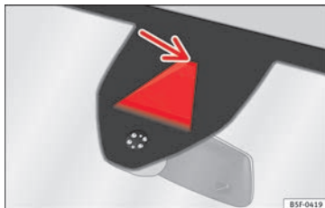
Fig. 193 In the windscreen: field of vision of the Lane Assist system camera.
