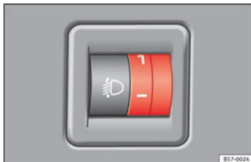
Fig. 138 Next to the steering wheel: Headlight range control
