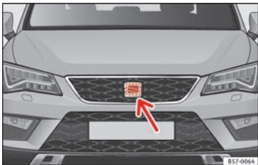
Fig. 179 On the front behind the SEAT badge: radar sensor.
