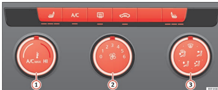
Fig. 56 In the centre console: Manual air conditioning controls
