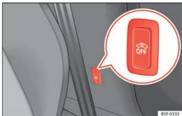
Fig. 130 Vehicle interior monitoring/tow-away protection button.
