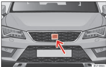
Fig. 187 On the front behind the SEAT badge: radar sensor.
