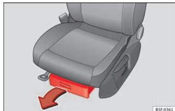
Fig. 147 Storage compartment under the front seats.
