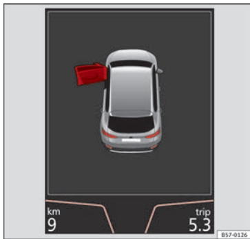
Fig. 50 On the instrument panel display: door open.
