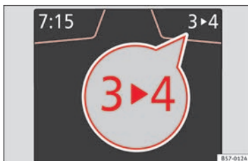
Fig. 45 Instrument panel: gear-change indicator (manual gearbox).
