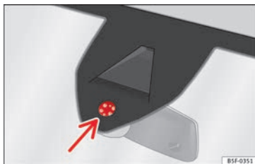
Fig. 141 Rain sensor sensitive surface
