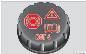
Fig. 62 Engine compartment: brake fluid reservoir cap
