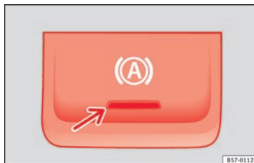
Fig. 172 In the lower part of the centre console: Auto Hold function button.
