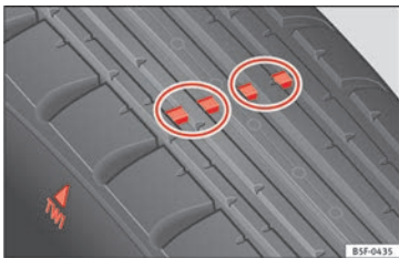
Fig. 227 Tyre tread: tread wear indicators
