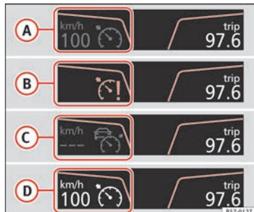
Fig. 173 Instrument panel display: CCS status indications
