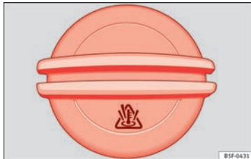
Fig. 61 Engine compartment: coolant expansion tank cap.
