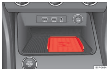
Fig. 122 Centre console: Connectivity Box
