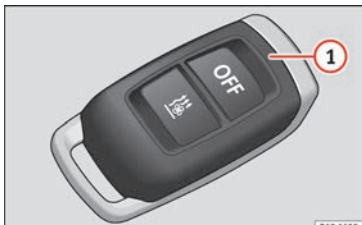
Fig. 164 Auxiliary heater: remote control.
