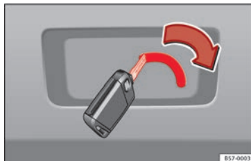
Fig. 8 Luggage compartment: emergency release.
