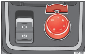
Fig. 199 Centre console: Driving Experience button.
