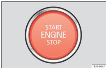
Fig. 166 In the lower part of the centre console: starter button.
