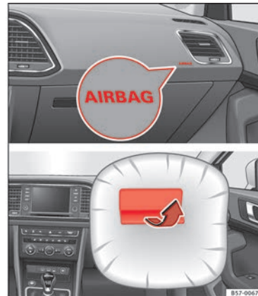
Fig. 21 Front passenger airbag located in dash panel.
