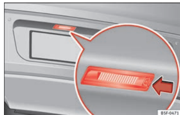
Fig. 114 In the rear bumper: number plate light.
