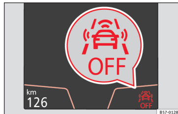
Fig. 188 On the instrument panel display: Front Assist switched off message.
