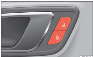
Fig. 2 Driver door: central locking switch.
