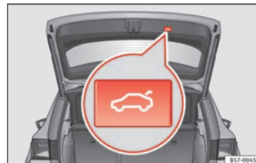
Fig. 6 Rear lid: button to close rear lid.
