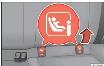
Fig. 31 ISOFIX/iSize securing rings.
