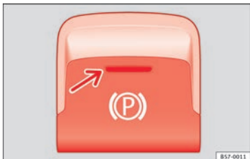
Fig. 167 In the lower part of the centre console: electronic parking brake button.
