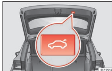
Fig. 131 Rear lid open: button to close the rear lid immediately.
