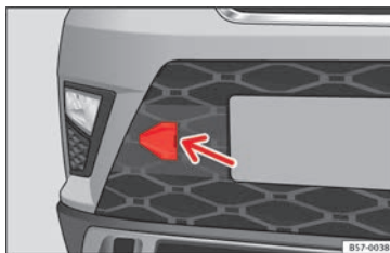
Fig. 97 Front bumper on right: remove the lid.
