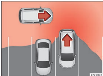
Fig. 198 Schematic representation of the rear cross traffic alert: monitored zone around the vehicle being parked.
