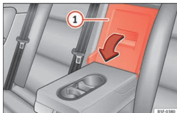
Fig. 154 On the rear seat backrest: opening the tailboard.
