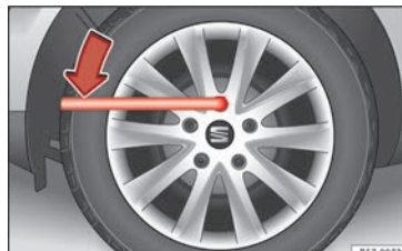
Fig. 72 Wheel: loosen the wheel bolts.
