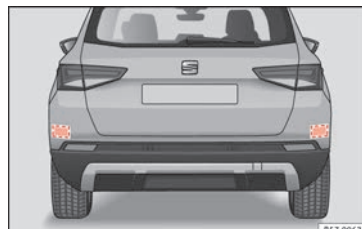
Fig. 195 Rear view of the vehicle: radar sensor zones.
