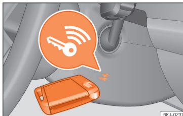
Fig. 242 On the right of the steering column: emergency start.
