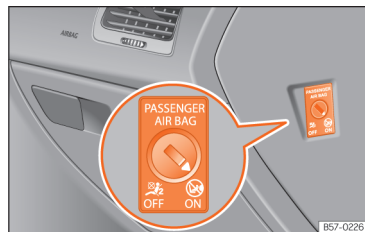
Fig. 98 Switch for activating and deactivating the front passenger airbag.
