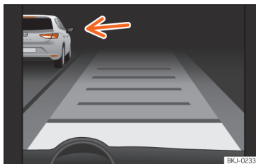
Fig. 263 On the instrument panel display: ACC active, vehicle detected in an outer lane.
