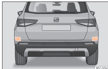
Fig. 272 Rear view of the vehicle: radar sensor areas.
