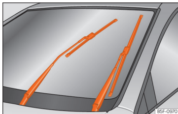
Fig. 84 Wipers in service position.
