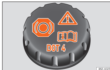
Fig. 65 Engine compartment: brake fluid reservoir cap.
