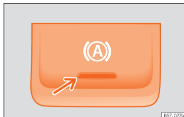
Fig. 249 In the lower part of the centre console: Auto Hold function button.
