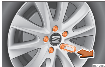
Fig. 75 Wheel: wheel bolts with caps.
