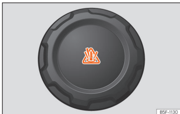
Fig. 64 Engine compartment: coolant expansion tank cap.
