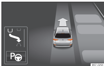
Fig. 281 On the instrument panel display: display of the assisted parking system with decreased visibility.
