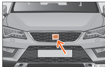
Fig. 260 On the front behind the SEAT badge: radar sensor.
