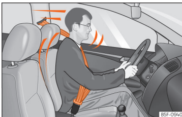
Fig. 93 Drivers with properly worn seat belts will not be thrown forward in the event of sudden braking.
