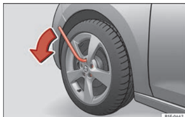
Fig. 64 Wheel: loosen the wheel bolts.
