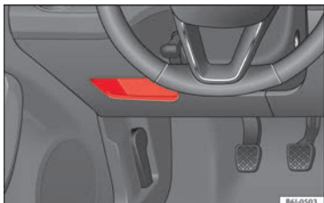
Fig. 56 On the driver-side dash panel: fuse box cover
