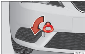
Fig. 87 Towline anchorage at the front of the vehicle
