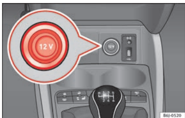
Fig. 146 Front power socket.
