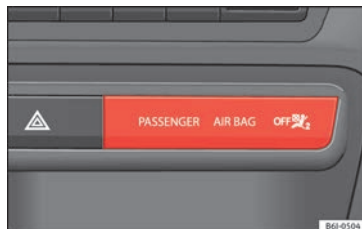
Fig. 85 Centre side of dash panel: control lamp for deactivated front passenger airbag in centre console
