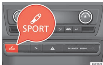
Fig. 171 In the centre console: button to adjust the “SEAT Drive Profile” system
