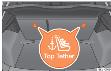
Fig. 35 Position of the Top Tether rings on the back of the rear seat.
