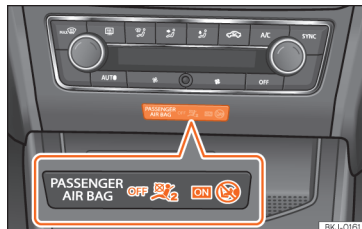
Fig. 97 Centre of the instrument panel: control lamp for deactivated front passenger airbag in centre console.
