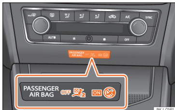
Fig. 26 Centre of the instrument panel: control lamp for deactivated front passenger airbag in centre console.
