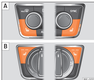
Fig. 151 On the centre console: front seats heating switch [A]: version with Climatronic. [B]: version with manual air conditioning.
