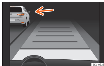
Fig. 240 On the instrument panel display: ACC active, vehicle detected in an outer lane.
