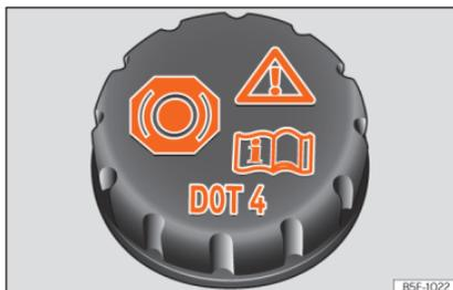
**Fig. 274** Engine compartment: brake fluid reservoir cap.
