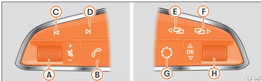
Fig. 83 Controls on the steering wheel.
