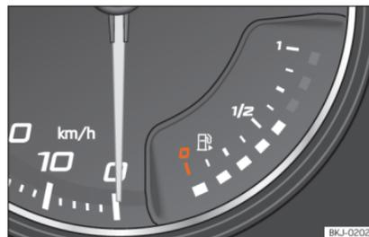
**Fig.72** Analogue instrument panel: fuel gauge
