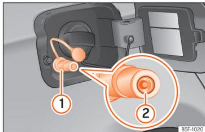
**Fig. 262** Tank cap open: gas filler mouth (1), filler mouth retainer (2).
