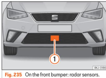
**Fig. 235** On the front bumper: radar sensors.
