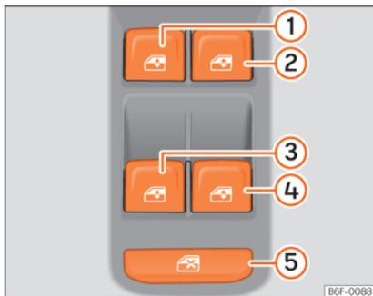
**Fig. 101** Detail of the driver's door: window controls.
