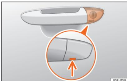
**Fig. 95** Driver door handle: Concealed lock cylinder.
