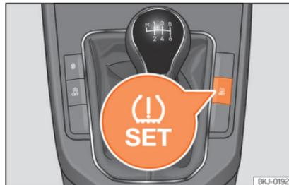
Fig. 279 Centre console: tyre pressure loss indicator button.
