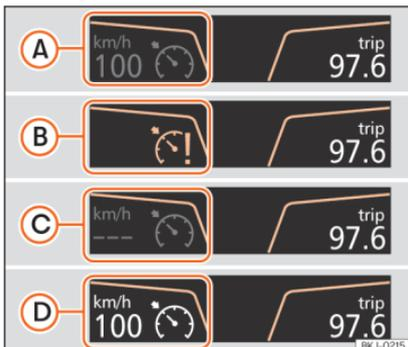
**Fig. 222** Instrument panel display: GRA status indications.
