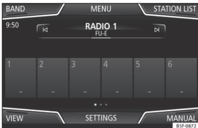
**Fig. 164** Display of memory buttons in DAB mode.
