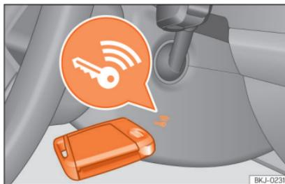
**Fig. 211** On the right of the steering column: emergency start.
