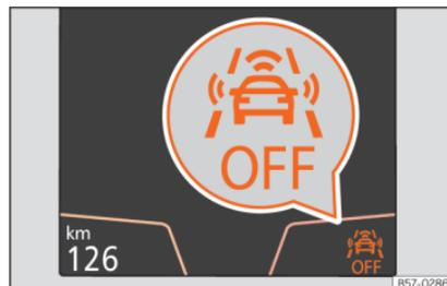
**Fig. 230** On the instrument panel display: Front Assist deactivated indication.
