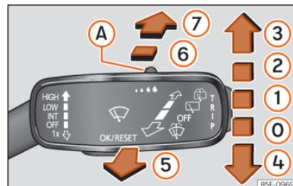
**Fig. 113** Operating the windscreen wiper and rear wiper.
