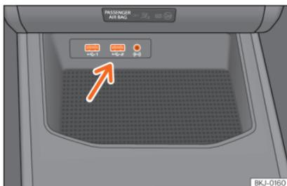
**Fig. 206** Centre console: USB/AUX-IN input.
