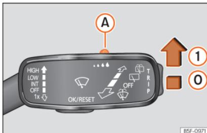
**Fig. 114** Wiper lever: adjust the rain sensor **A**
