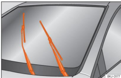
**Fig. 42** Wipers in service position.
