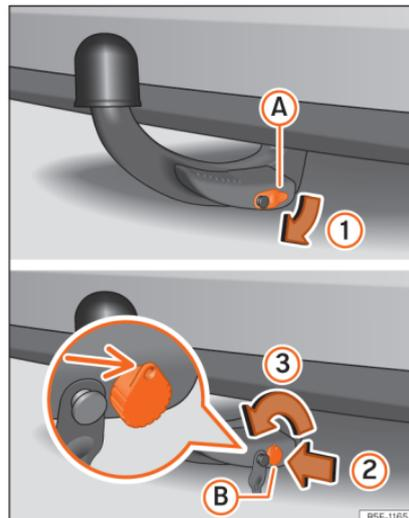
**Fig. 257** Removing the tow hook
