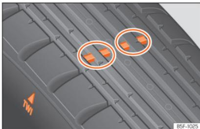
**Fig. 277** Tyre profile: tread wear indicators.
