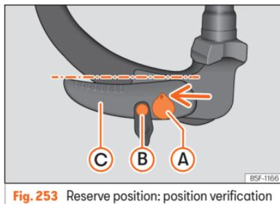
Before assembling it, place the tow hook in the standby position with the following two steps.
