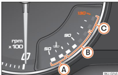
**Fig. 75** Analogue instrument panel: engine coolant temperature indicator.
