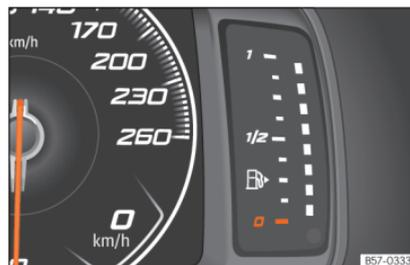
**Fig.73** Digital instrument panel: fuel gauge.
