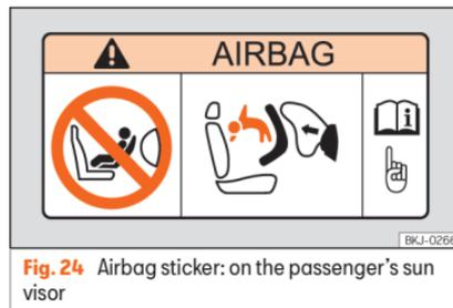
**Fig. 24** Airbag sticker: on the passenger's sun visor
