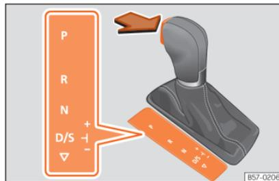
Fig. 215 Selector lever lock.
