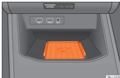
**Fig. 208** In the centre console: pad for the mobile phone connection.
