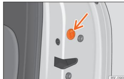
**Fig. 97** Locking the door manually. »
