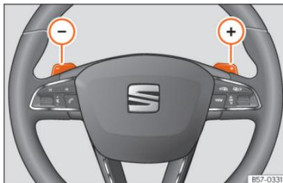
**Fig. 217** Steering wheel: automatic transmission levers
