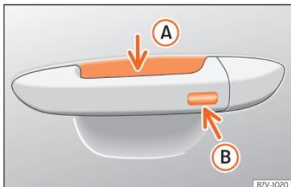
Fig. 94 Door handle: sensor surfaces
