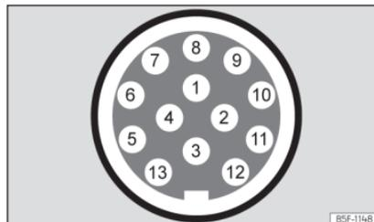
**Fig. 250** Schematic representation: assignment of the pins of the trailer's electrical socket.
