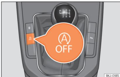
**Fig. 213** Centre console: Start-stop system button.
