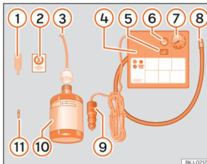
**Fig. 32** Standard representation: anti-puncture kit contents.
