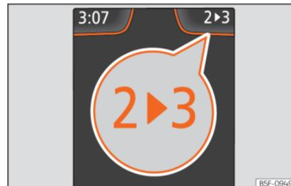
**Fig. 219** Instrument panel: gear-change indicator (manual gearbox).
