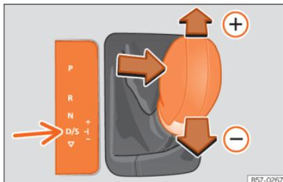
**Fig. 216** Lever in the Tiptronic position
