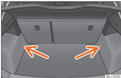
**Fig. 130** Location of fastening rings in luggage compartment.
