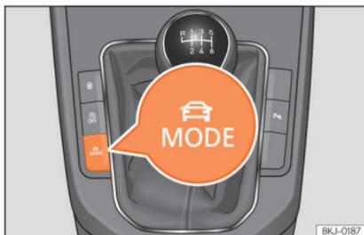
**Fig. 220** Next to the gear lever: MODE button.
