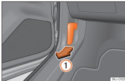
**Fig. 267** Release lever in the driver's footwell area.
