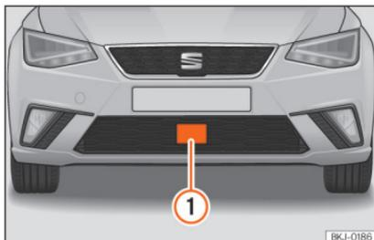
**Fig. 229** On the front bumper: radar sensors.
