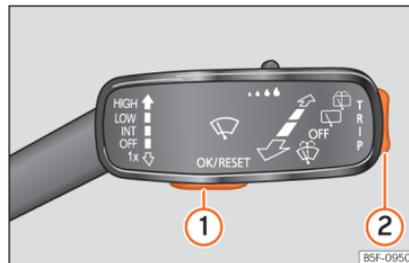
Fig.77 Wiper lever: control keys.
