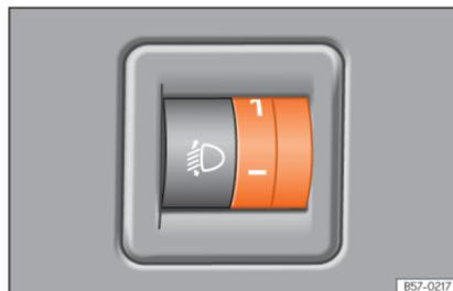
**Fig. 110** Next to the steering wheel: headlight range control.
