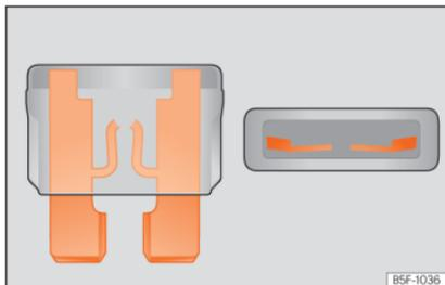
**Fig. 53** Image of a blown fuse.
