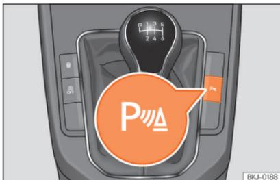
**Fig. 244** Centre console: parking aid button (depending on the version).
