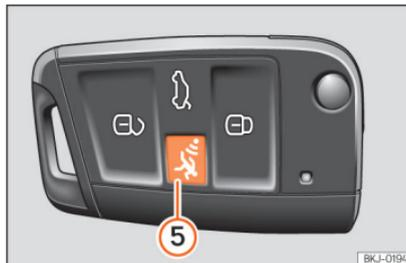
**Fig. 86** Vehicle key with alarm button.
