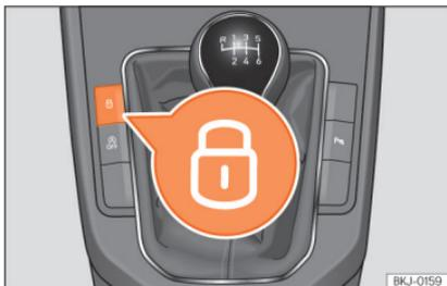
**Fig. 90** Centre console: central locking button.
