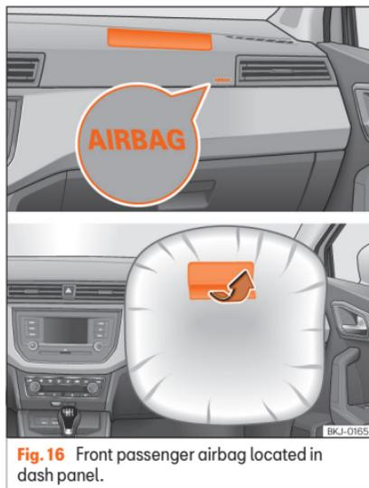
**Fig. 16** Front passenger airbag located in dash panel.
