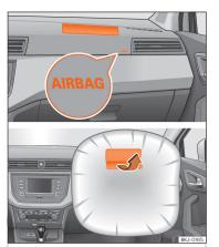
Fig. 16 Front passenger airbag located in dash panel.
