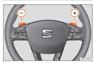
Fig. 217 Steering wheel: automatic transmission levers
