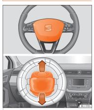
Fig. 15 Driver airbag located in steering wheel.
