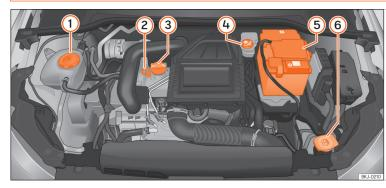
From time to time, the levels of the different fluids in the vehicle must be checked. Never fill with incorrect fluids, otherwise serious damage to the engine may be caused.
