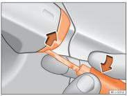
Fig. 96 Driver door handle: lever the cover off
