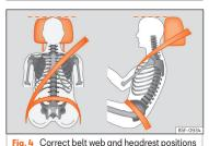
Fig. 4 Correct belt web and neadrest positions
