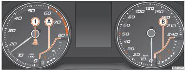
Fig. 74 Analogue instrument panel: natural gas gauge
