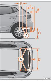
**Fig. 260** Limits and attachment points for retrofitting a towing bracket.
