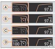
**Fig. 222** Instrument panel display: GRA status indications.
