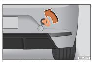
**Fig. 50** Right side of the rear bumper: towline anchorage in position.
