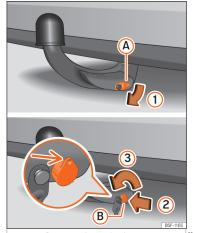
Fig. 257 Removing the tow hook
