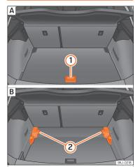
**Fig. 128** Variable luggage compartment floor: A raised position; B lowered position.
