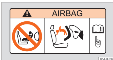
Fig. 22 Airbag sticker: on the passenger's sun visor
