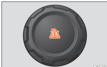
Fig. 192 Engine compartment: coolant expansion tank cap.
