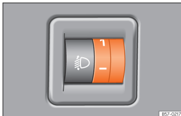
Fig. 99 Next to the steering wheel: headlight range control.
