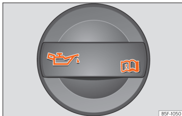
Fig. 190 In the engine compartment: Engine oil filler cap.
