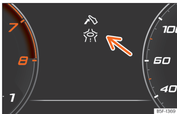
Fig. 65 Eco-efficient driving assistance indication (schematic representation).
