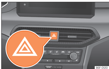
Fig. 98 Dash panel: hazard warning lights switch
