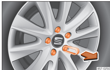
Fig. 34 Wheel: wheel nuts with caps.
