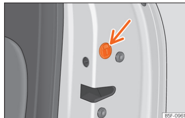
Fig. 88 Locking the door manually.
