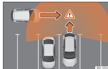
Fig. 164 Schematic representation of the rear cross traffic alert assistant: zone monitored around the vehicle while leaving a parking space.
