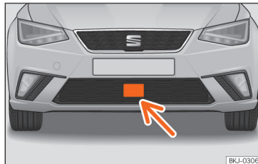
Fig. 142 On the front bumper: radar sensors.
