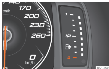
Fig. 67 Digital instrument panel: fuel gauge. »
