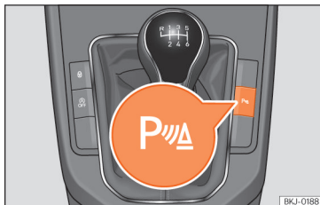
Fig. 167 Centre console: parking aid button (depending on the version).
