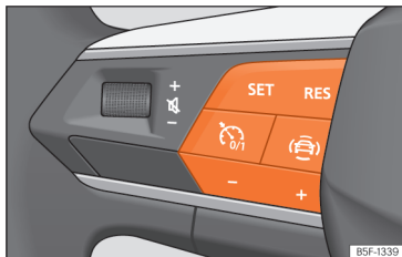
Fig. 148 On the multifunction steering wheel: buttons to operate the speed limiter.
