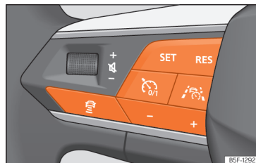
Fig. 160 Left side of the multifunction steering wheel: buttons for operating Travel Assist.
