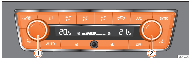
Fig. 122 In the centre console: Climatronic controls.
