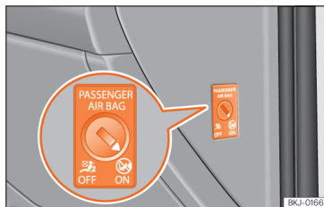
Fig. 16 Switch for activating and deactivating the front passenger airbag.
