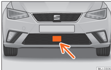
Fig. 142 On the front bumper: radar sensors.
