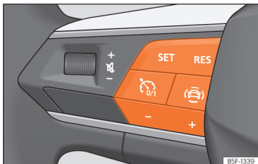
Fig. 149 On the multifunction steering wheel: buttons to operate the speed limiter.
