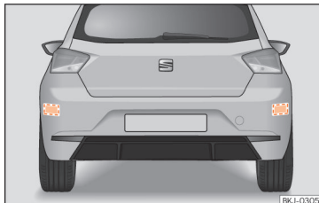
Fig. 145 Rear view of the vehicle: radar sensor zones.
