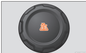
Fig. 193 Engine compartment: coolant expansion tank cap.
