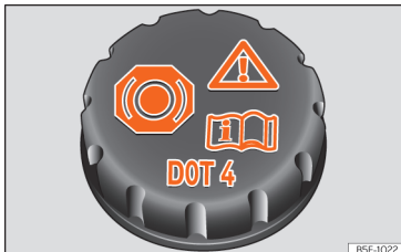
Fig. 194 Engine compartment: brake fluid reservoir cap.
