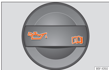
Fig. 178 Oil filler cap cover in the engine compartment.
