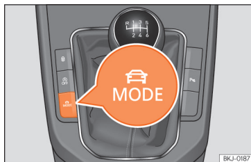
Fig. 93 Next to the gearbox lever: MODE button.
