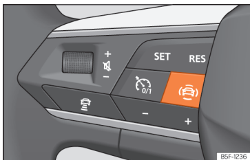
Fig. 95 Left side of the multifunction steering wheel: button for driver assistance systems (depending on the version).
