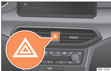
Fig. 44 Dashboard: switch for hazard warning lights.
