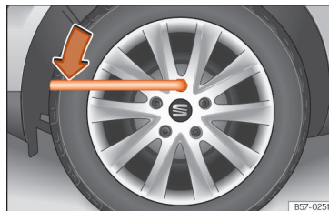
Fig. 188 Tyre change: slacken the wheel bolts.
