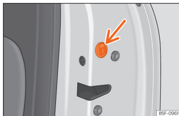
Fig. 56 Locking the door manually.
