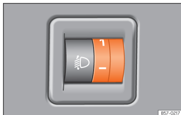
Fig. 75 Next to the steering wheel: regulator headlight range control.
