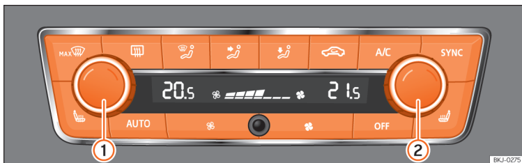
Fig. 82 In the centre console: Climatronic control panel.
