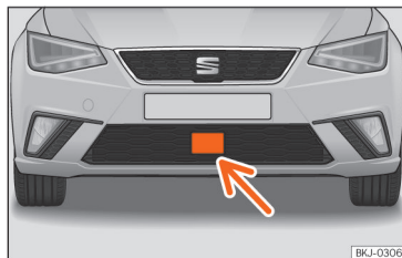
Fig. 96 On the front bumper: radar sensor.
