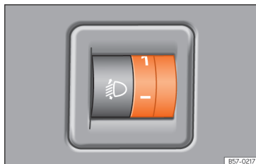
Fig. 74 Next to the steering wheel: regulator headlight range control.
