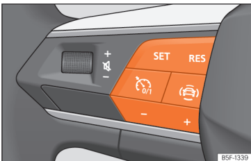
Fig. 102 On the multifunction steering wheel: cruise control operation buttons.
