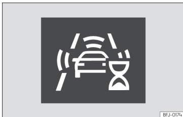
Fig. 110 On the instrument cluster screen: indication of the system's initial self-calibration.
