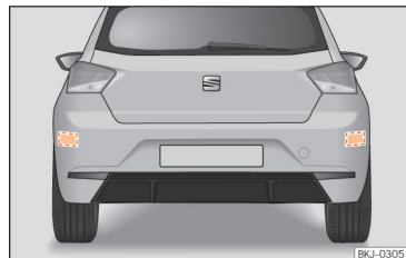
Fig. 99 Rear view of the vehicle: radar sensor areas.
