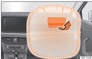
Fig. 28 Front passenger airbag located in dash panel.
