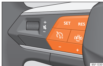
Fig. 103 On the multifunction steering wheel: buttons to control the speed limiter.
