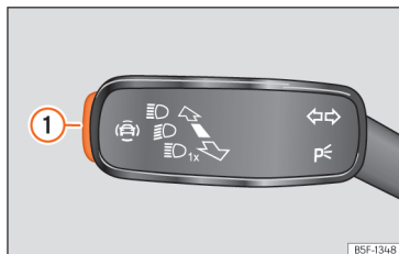
Fig. 94 On the turn light and main beam lever: key for driver assistance systems (depending on the version).
