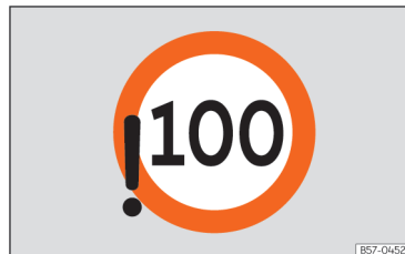
Fig. 11 On the instrument cluster screen: violation of the detected speed limit (illustration).
