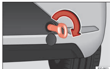
Fig. 76 Right side of the rear bumper: towline anchorage screwed in.
