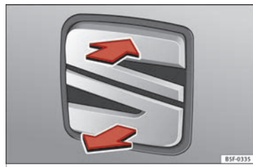
Fig. 5 Rear lid: opening from the outside.
