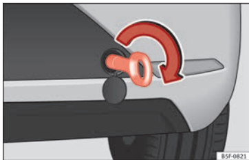
Fig. 99 Right side of the rear bumper: towline anchorage screwed in.
