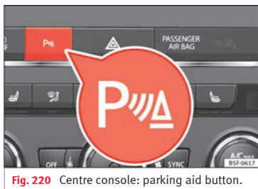
Fig. 220 Centre console: parking aid button.
