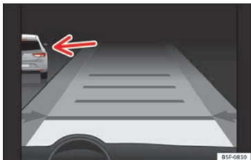
Fig. 204 On the instrument panel display: ACC active, vehicle detected in an outer lane
