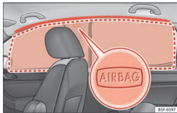
Fig. 27 Location of head-protection airbags.
