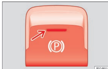
Fig. 188 In the lower part of the centre console: electronic parking brake button.
