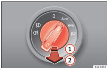
Fig. 138 Dash panel: light control.
