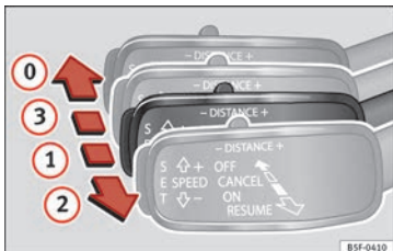
Fig. 200 On the left of the steering column: third lever for operating the Adaptive Cruise Control.
