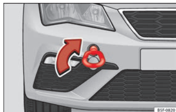
Fig. 97 Right side of the front bumper: towline anchorage screwed in.
