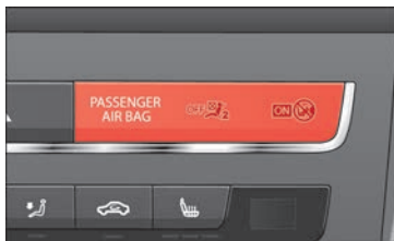
Fig. 93 Control lamp for disabling the front passenger front airbag on the dash panel
