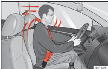
Fig. 88 Drivers with properly worn seat belts will not be thrown forward in the event of sudden braking
