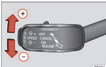
Fig. 201 On the left of the steering column: third lever for operating the Adaptive Cruise Control.
