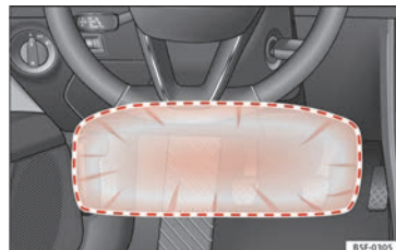
Fig. 24 On the driver side: radius of action of the knee airbag.
