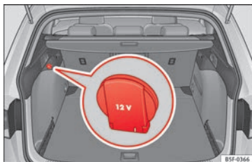
Fig. 158 Detailed view of the side trim in the luggage compartment: 12-volt power socket (applies only to the LEON ST model).
