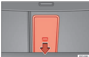
Fig. 172 In the luggage compartment: opening the tailboard.
