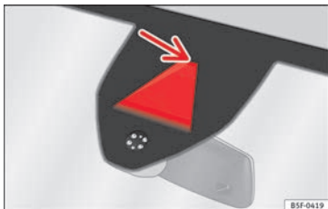
Fig. 214 In the windscreen: field of vision of the Lane Assist system camera.
