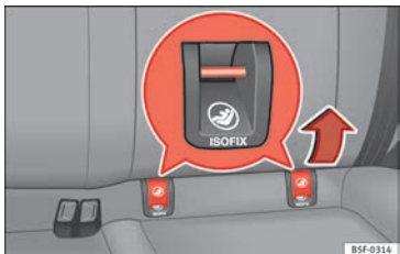
Fig. 31 ISOFIX securing rings.
