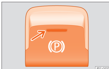
Fig. 285 In the lower part of the centre console: electronic parking brake button
