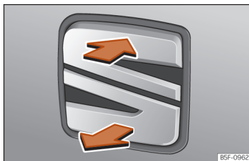
Fig. 105 Rear lid: opening from outside.
