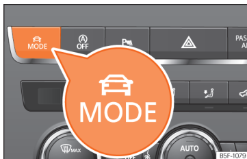
Fig. 264 Centre console: MODE button. You can select from Normal, Sport, Eco, Comfort and Individual.
