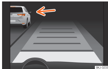
Fig. 278 On the instrument panel display: ACC active, vehicle detected in an outer lane.
