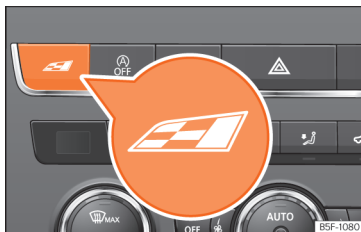
Fig. 265 Centre console: Cupra Drive Profile button. You can select from Comfort, Sport, Cupra and Individual
