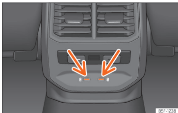
Fig. 165 Rear centre console: USB connectors with power socket function.
