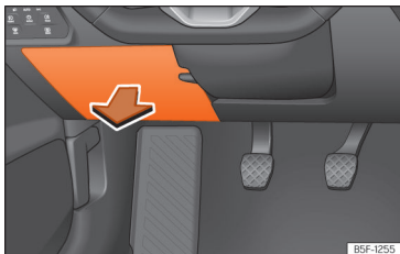
Fig. 215 On the dashboard on the driver side: lid of the fuse box.
