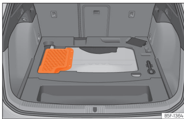
Fig. 229 Hybrid vehicles (PHEV): location of the battery in the luggage compartment
