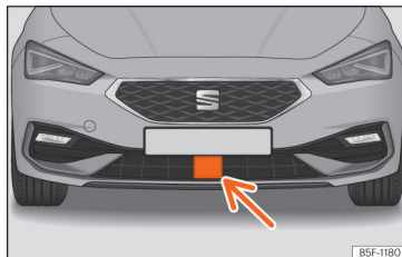
Fig. 122 On the front bumper: radar sensor.
