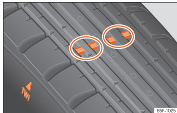
Fig. 233 Tyre profile: tread wear indicators.
