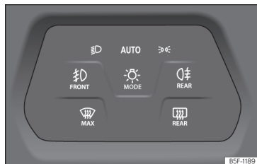
Fig. 101 Instrument panel: light panel.
