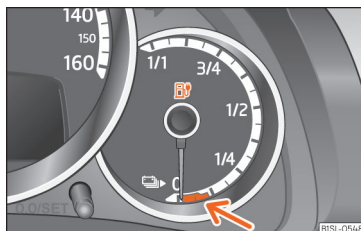
Fig. 149 On the instrument panel: indicator of the high-voltage battery charge level with the reserve area marked in red (arrow).
