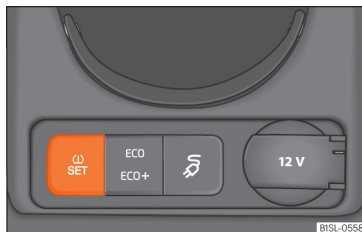
Fig. 169 Centre console: tyre monitoring system button.
