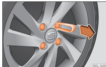
Fig. 31 Wheel: wheel bolts with caps.
