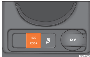
Fig. 139 At the bottom of the centre console: button for selecting the driving profile.
