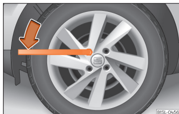
Fig. 33 Tyre change: slacken the wheel bolts.
