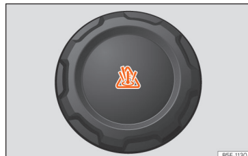
Fig. 162 Engine compartment: coolant expansion tank cap.
