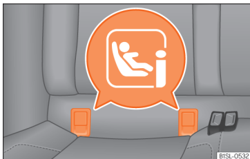
Fig. 23 Rear seat: ISOFIX/i-Size securing rings.
