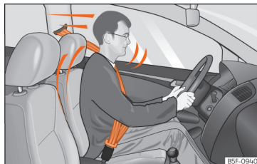
Fig. 6 Drivers with properly worn seat belts will not be thrown forward in the event of sudden braking.
