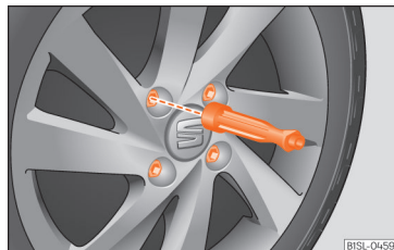
Fig. 37 Changing the tyre: loosen wheel bolts with the socket at the end of the wheel brace
