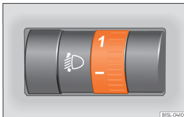
Fig. 82 Next to the steering wheel: regulator headlight range control.
