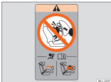
Fig. 22 Airbag sticker: on the rear frame of the passenger side door
