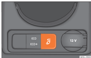
Fig. 151 At the bottom of the centre console: charging mode button.
