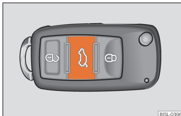
Fig. 73 On the vehicle key: button to unlock and open the boot hatch.
