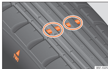
Fig. 167 Tyre profile: tread wear indicators.
