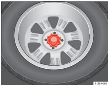
Fig. 177 In the luggage compartment: hand controlled wheel for securing the spare wheel
