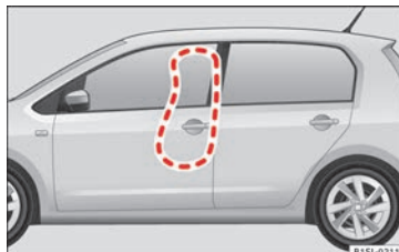
Fig. 22 On the left side of the vehicle: deployment area of side airbag
