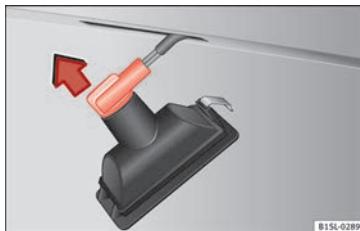
Fig. 91 Number plate light: Remove the bulb holder.
