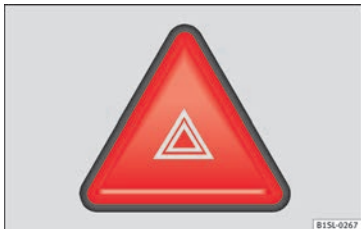
Fig. 110 Dash panel: Button for switching the hazard lights warning system on and off.
