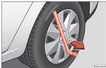
Fig. 51 Removing the full hubcap
