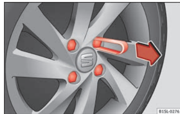
Fig. 52 Removing the wheel bolt caps
