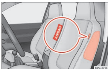
Fig. 21 On the side of the front seat: location of the side airbag
