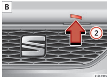
Fig. 8 A: Release lever in the footwell on the driver side B: Release lever on the bonnet
