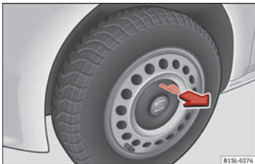
Fig. 50 Remove the hubcap of the steel wheel trim
