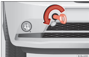
Fig. 81 On the right-hand side of the front bumper: Screw in the towline anchorage.
