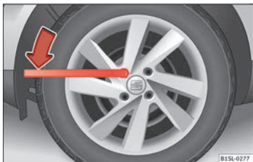
Fig. 53 Changing a wheel: Slacken the wheel bolts.
