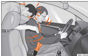
Fig. 72 The unbelted passenger in the rear seat is thrown forward violently, hitting the driver who is wearing a seat belt.
