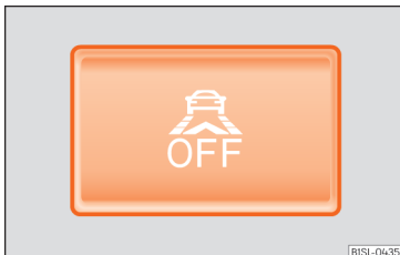
Fig. 171 In the lower part of the centre console: button for the city safety assist function.
