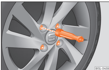
Fig. 58 Changing the tyre: loosen wheel bolts with the socket at the end of the wheel brace
