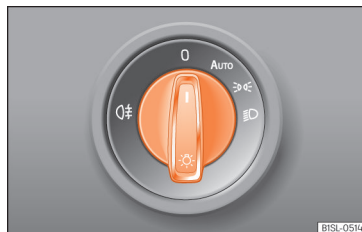
Fig. 110 On the side of the steering wheel: diagram of some of the types of light switch
