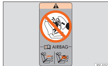
Fig. 25 On the rear frame of the passenger side door: adhesive in relation to the airbag.
