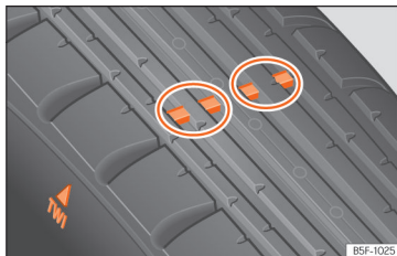
Fig. 188 Tyre profile: tread wear indicators.
