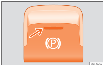
Fig. 193 In the lower part of the centre console: electronic parking brake button
