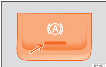
Fig. 194 In the lower part of the centre console: Auto Hold function button.
