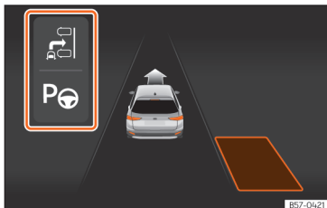
Fig. 196 On the instrument panel display: view of the parking assist system with reduced view.
