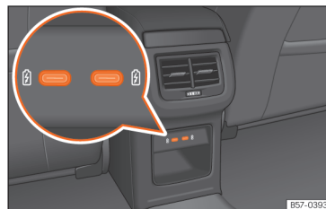
Fig. 156 Rear part of the centre console: USB connectors with power outlet function.
