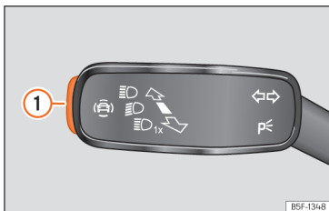
Fig. 77 On the turn signal and main beam lever: button for driver assistance systems (depending on versions).
