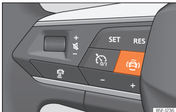
Fig. 78 Left side of the multifunction steering wheel: button for driver assistance systems (depending on versions).
