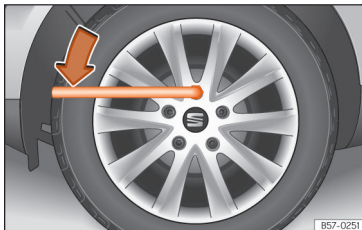
Fig. 36 Wheel change: loosen the wheel nuts.
