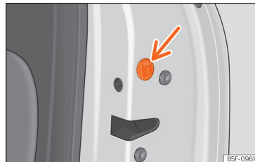
Fig. 95 Locking the door manually.
