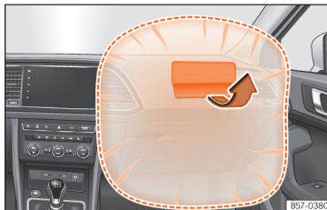
Fig. 15 Front passenger airbag located in dash panel.
