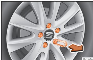
Fig. 34 Wheel: wheel nuts with caps.
