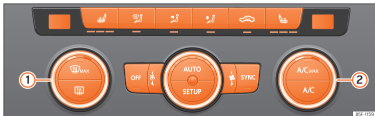
Fig. 134 In the centre console: Climatronic controls.
