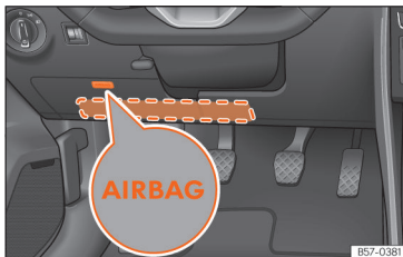
Fig. 18 On the driver side: location of the knee airbag
