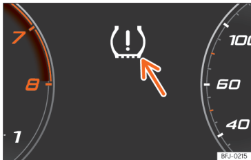
Fig. 221 Instrument panel: warning of loss of tyre pressure.
