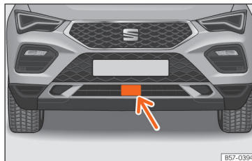
Fig. 157 On the front bumper: radar sensors.
