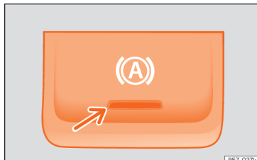
Fig. 183 In the lower part of the centre console: Auto Hold function button.
