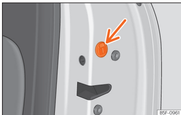
Fig. 84 Locking the door manually.
