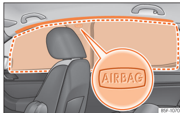
Fig. 22 Location of head-protection airbags.
