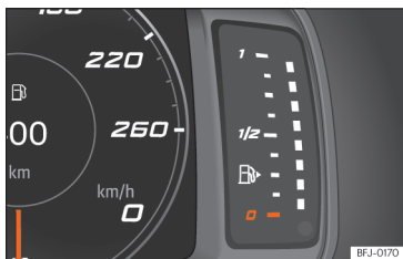
Fig. 60 Digital instrument panel: fuel gauge.
