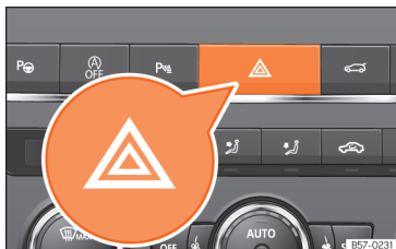
Fig. 99 Dash panel: hazard warning lights switch
