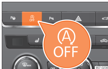
Fig. 150 Centre console: Start-stop system button.
