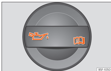
Fig. 213 In the engine compartment: Engine oil filler cap.
