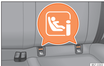
Fig. 26 Rear seat: ISOFIX/i-Size securing rings.
