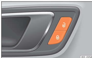
Fig. 79 Driver's door: central locking switch.
