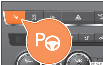
Fig. 184 In the upper part of the centre console: button to switch on the Park Assist system.
