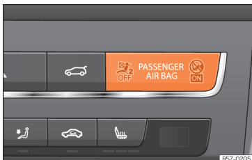
Fig. 17 Dash panel: control lamp for the deactivation of the front passenger front airbag.
