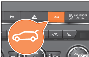
Fig. 88 Centre console: button to open and close the rear lid.
