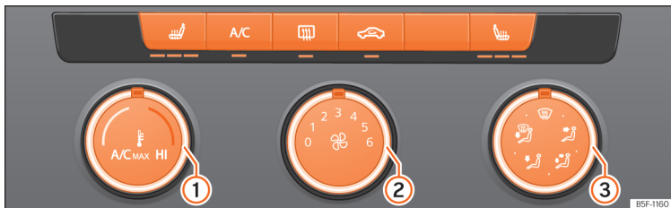
Fig. 135 In the centre console: Manual air conditioning controls.
