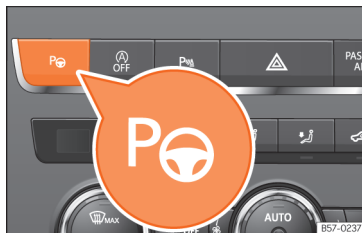
Fig. 137 In the centre console, top section: button to switch on the Park Assist system.
