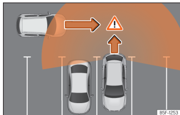
Fig. 149 Diagram of the parking assistant: detected area around the vehicle that is driving off.
