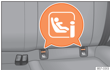
Fig. 39 Rear seat: location of the ISOFIX or i-Size securing rings.
