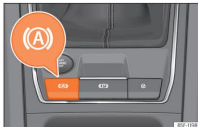
**Fig. 164** In the lower part of the centre console: Auto Hold function button.
