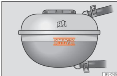
**Fig. 185** In the engine compartment: marking on coolant expansion tank.
