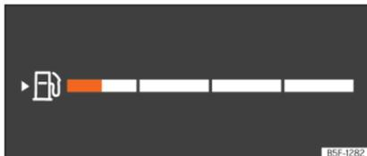
**Fig. 57** Digital instrument panel: fuel level indicator located in different positions depending on the view.
