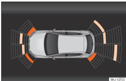
**Fig. 171** Parking Aid display on the Infotainment system screen.
