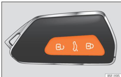
**Fig. 72** Remote control key: buttons.
