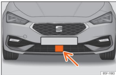
**Fig. 142** On the front bumper: radar sensors.
