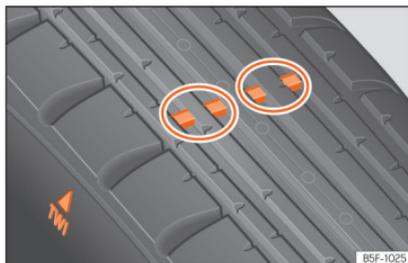
**Fig. 190** Tyre profile: tread wear indicators.
