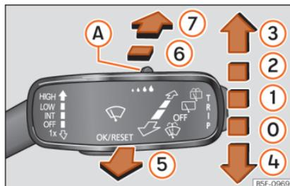
**Fig. 89** Operating the windscreen wiper and rear wiper.
