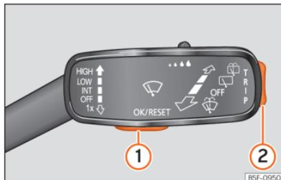
Fig. 59 Wiper lever: control keys.
