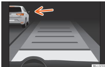
**Fig. 147** On the instrument panel display: ACC active, vehicle detected in an outer lane.
