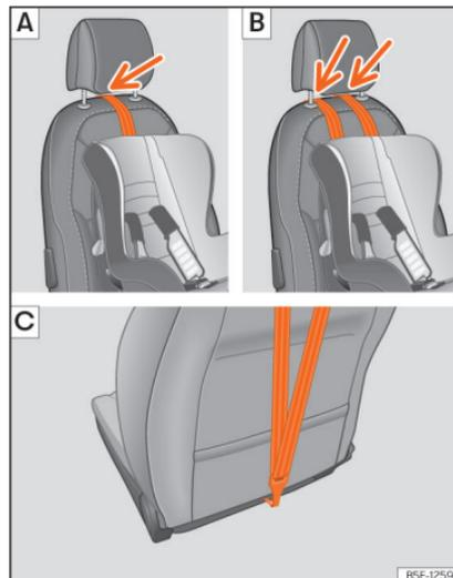
**Fig. 28** Front passenger seat: adjustment and assembly according to the Top Tether belt.
