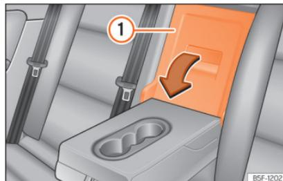
**Fig. 109** In the rear seat backrest: opening the trapdoor.
