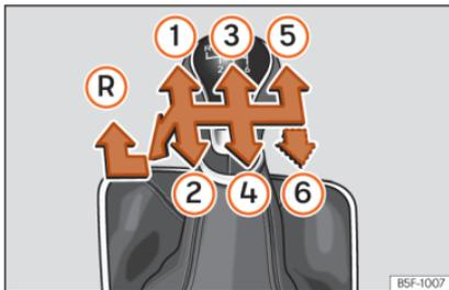
**Fig. 131** Gear shift pattern of a 5 or 6-speed manual gearbox.
