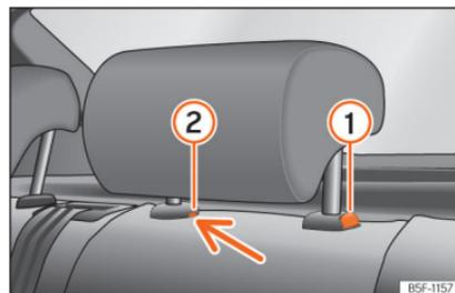
**Fig. 97** Rear headrest: removal.
