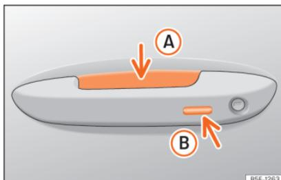
**Fig. 75** Door handle: sensor surfaces
