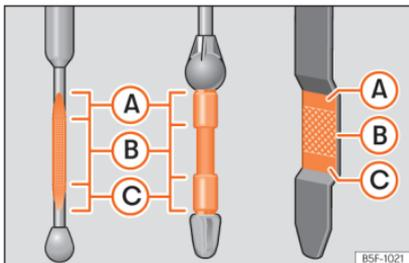
**Fig. 183** Engine oil dipstick.
