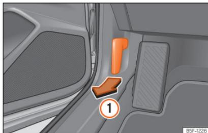
**Fig. 180** Release lever in the driver's footwell area.
