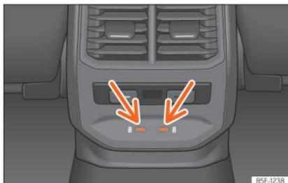
**Fig. 116** Back of the centre console: USB power sockets.
