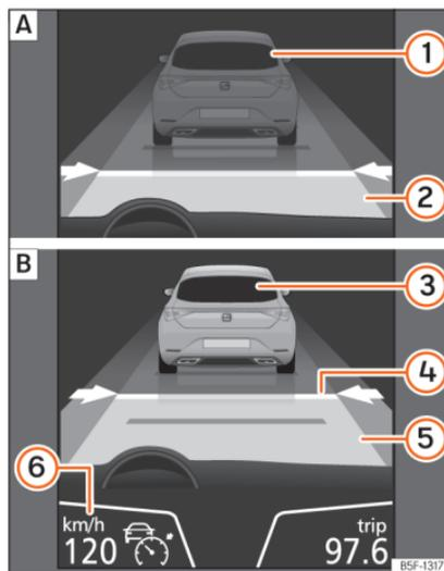
**Fig. 144** On the instrument panel display: **A** ACC inactive (Standby). **B** ACC active.
