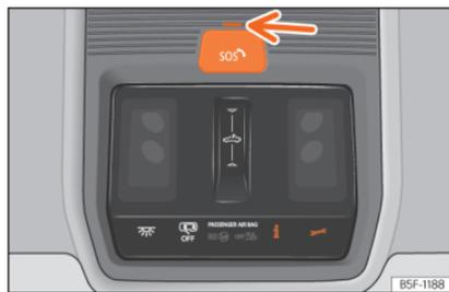
**Fig. 30** On the roof console: voice service controls
