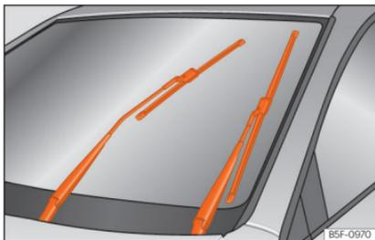
**Fig. 40** Wipers in service position.
