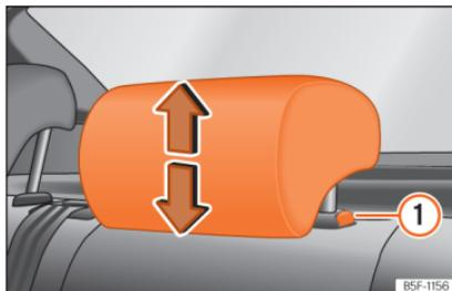
**Fig. 96** Rear headrest: headrest adjustment.
