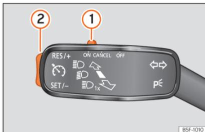
**Fig. 136** On the turn signal lever: controls for operating the GRA.
