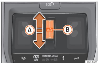
**Fig. 82** On the interior roof lining: sunroof button.
