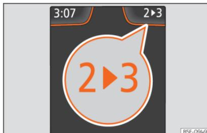
**Fig. 134** Instrument panel: gear-change indicator (manual gearbox).
