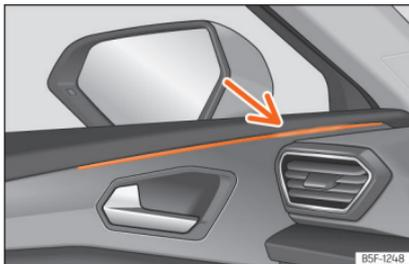
**Fig. 155** Control lamp of the lane departure warning.
