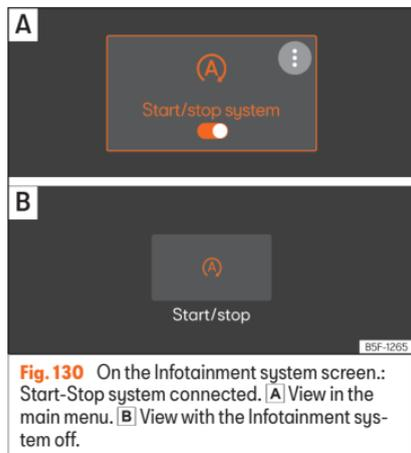
**Fig. 130** On the Infotainment system screen: Start-Stop system connected. **[A]** View in the main menu. **[B]** View with the Infotainment system off.
