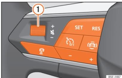
Fig. 67 Controls on the steering wheel.
