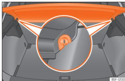
**Fig. 102** In the luggage compartment: removing and fitting the shelf.
