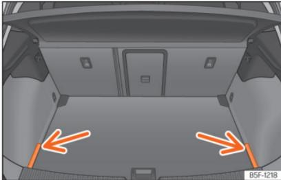
**Fig. 103** In the luggage compartment: covers for storing the rear shelf.
