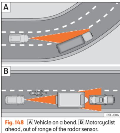
**Fig. 148** **A** Vehicle on a bend. **B** Motorcyclist ahead, out of range of the radar sensor.
