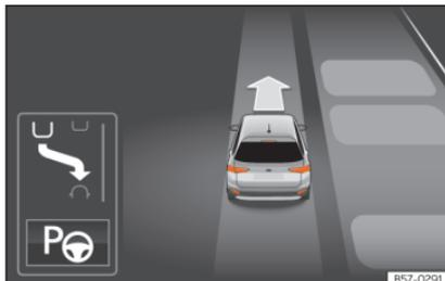
**Fig. 165** On the instrument panel display: view of the parking assist system with reduced view.
