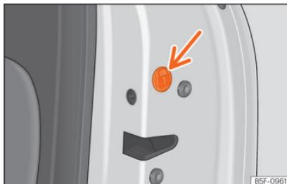
**Fig. 77** Locking the door manually.
