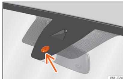
**Fig. 91** Rain sensor sensitive surface
