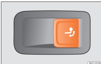
**Fig. 175** On the left side of the luggage compartment: button for unlocking the tow hook.
