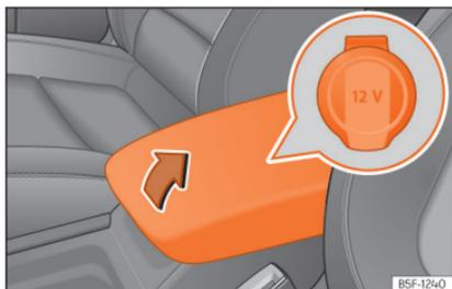
**Fig. 115** In the front armrest: 12 volt power socket.
