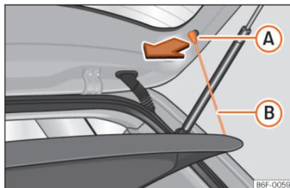
**Fig. 101** In the luggage compartment: removing and fitting the shelf.
