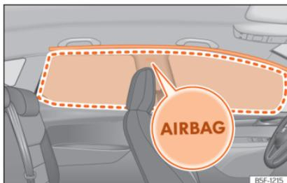
**Fig. 21** Location of head-protection airbags.
