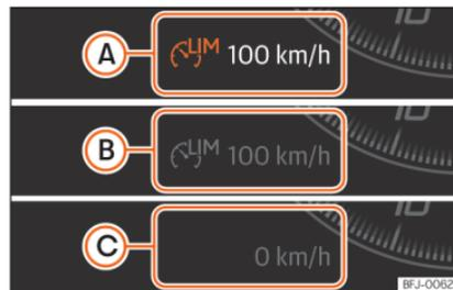
Fig. 137 On the instrument panel display: indications of the speed limited status.
