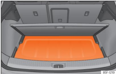
**Fig. 104** In the luggage compartment: fitting the rear shelf.
