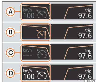
**Fig. 135** Instrument panel display: GRA status indications.
