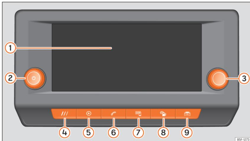
**Fig. 120** Overview: control unit and indication in the 8.25-inch version
