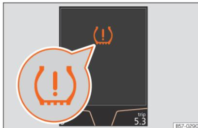
**Fig. 192** Instrument panel: warning of loss of tyre pressure.
