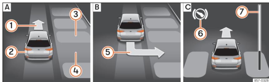
**Fig. 168** On the instrument panel display: angle parking. **A** Finding a parking space. **B** Parking position. **C** Manoeuvring.
