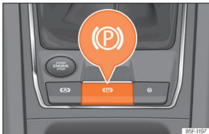
**Fig. 163** In the lower part of the centre console: electronic parking brake button
