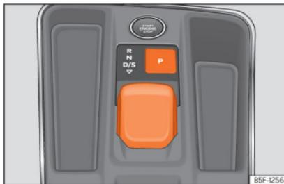
**Fig. 132** In the centre console: selector lever.
