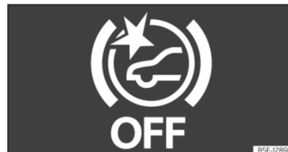
**Fig. 141** On the instrument panel display: Front Assist deactivated indication.
