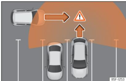
**Fig. 160** Schematic representation of the rear cross traffic alert assistant: zone monitored around the vehicle while leaving a parking space.
