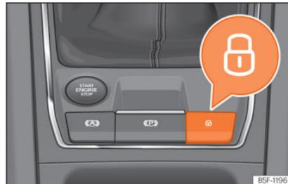
**Fig. 73** In the centre console: central locking switch
