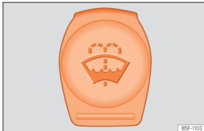
**Fig. 188** In the engine compartment: window washer tank cap.
