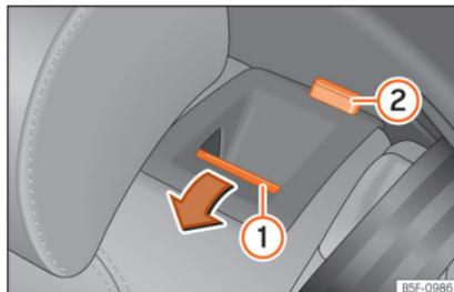
**Fig. 99** Rear seat: folding the backrest.
