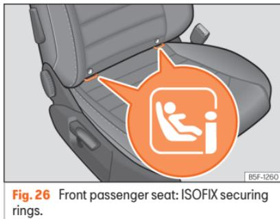
**Fig. 26** Front passenger seat: ISOFIX securing rings.
