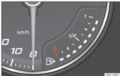
**Fig. 56** Analogue instrument panel: fuel gauge
