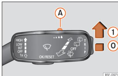
**Fig. 90** Wiper lever: adjust the rain sensor (A)
