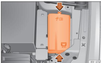
**Fig. 49** In the engine compartment: fuse box cover.
