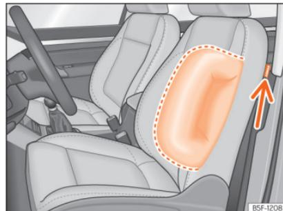
**Fig. 19** Side airbag in driver's seat.
