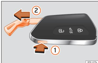
Fig. 70 Vehicle key: remove the key blade.
