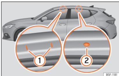
**Fig. 111** Attachment points for the roof railings for the roof carrier system.
