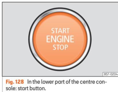
**Fig. 128** In the lower part of the centre console: start button.
