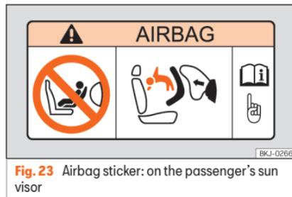
**Fig. 23** Airbag sticker: on the passenger's sun visor
