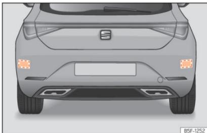
**Fig. 157** Rear view of the vehicle: radar sensor zones.
