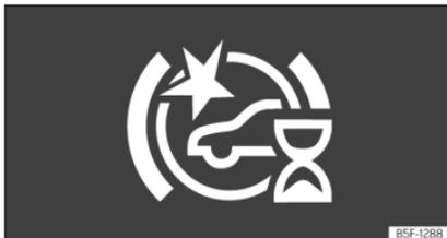
**Fig. 140** On the instrument panel display: initial system self-calibration indication.
