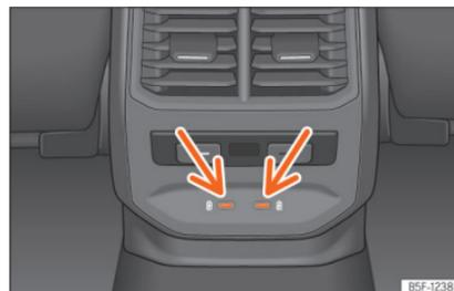
Fig. 127 Rear part of the centre console: USB connectors with power outlet function.
