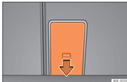
**Fig. 110** In the luggage compartment: opening the trapdoor.
