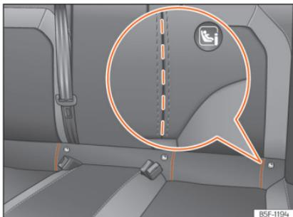
**Fig. 25** Rear seat: cut-out grooves to access the ISOFIX securing rings.
