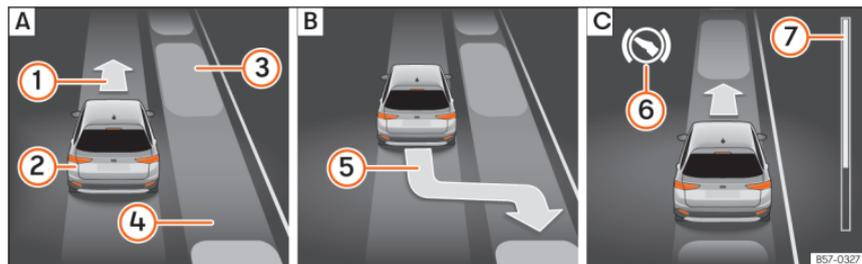
**Fig. 167** On the instrument panel display: parallel parking. **A** Finding a parking space. **B** Parking position. **C** Manoeuvring.
