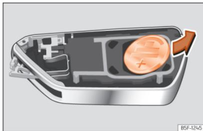
**Fig. 71** Vehicle key: removing the battery.
