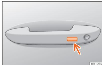
**Fig. 83** Door handle: sensor surface.
