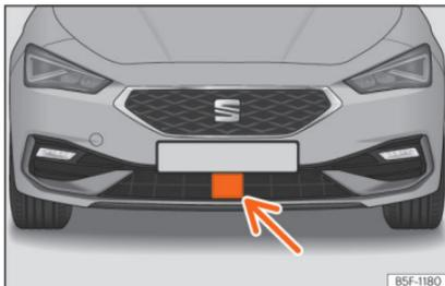
**Fig. 145** On the front bumper: radar sensors.
