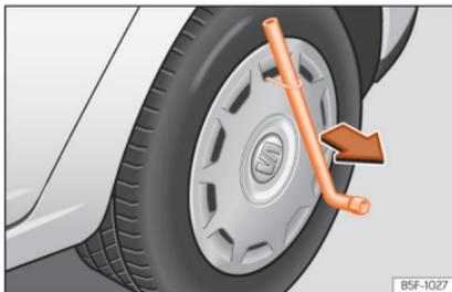
**Fig. 33** Remove the wheel cover.
