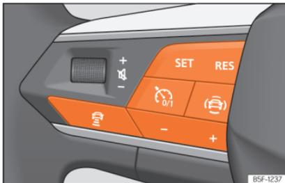
**Fig. 146** On the multifunction steering wheel: buttons to operate the ACC
