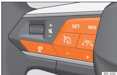
**Fig. 154** Left side of the multifunction steering wheel: buttons for operating Travel Assist.
