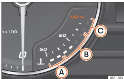
**Fig. 58** Analogue instrument panel: engine coolant temperature indicator.
