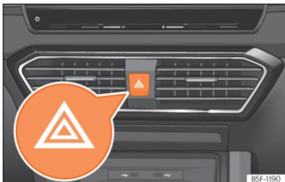
**Fig. 86** Dash panel: hazard warning lights switch
