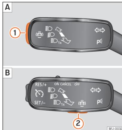
**Fig. 61** On the turn signal and main beam lever: button for driver assistance systems (depending on versions).
