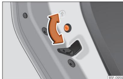
**Fig. 78** Childproof lock on the left hand side door.
