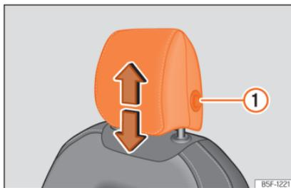
**Fig. 95** Front seat: headrest adjustment.
