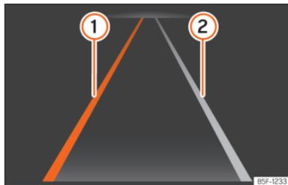
**Fig. 151** On the instrument panel display: indications of the Lane Assist System.
