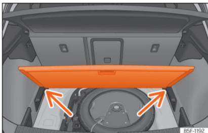
**Fig. 106** Variable luggage compartment floor: inclined position.
