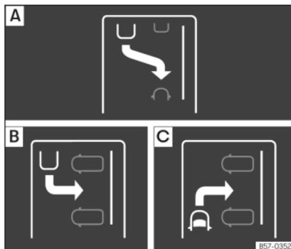
**Fig. 166** On the instrument panel display: indication of parking modes.
