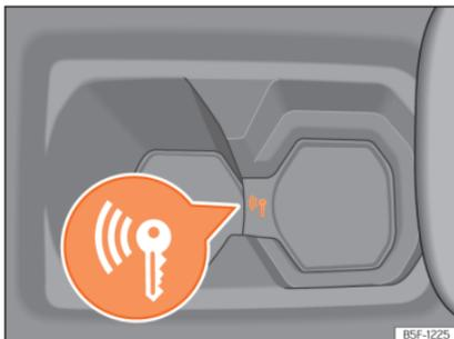
**Fig. 129** In the centre console: emergency start.
