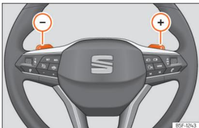
**Fig. 133** Steering wheel: automatic transmission levers
