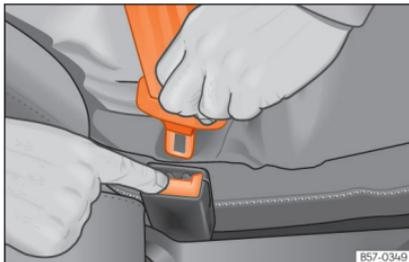
**Fig. 10** Release the seat belt's buckle.
