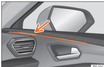
**Fig. 156** Control lamp of the lane departure warning.
