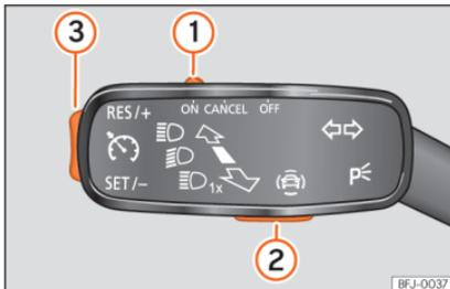
**Fig. 138** On the turn signal lever: buttons to operate the speed limiter.
