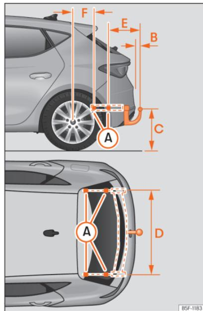
**Fig. 176** Limits and attachment points for retrofitting a towing bracket.
