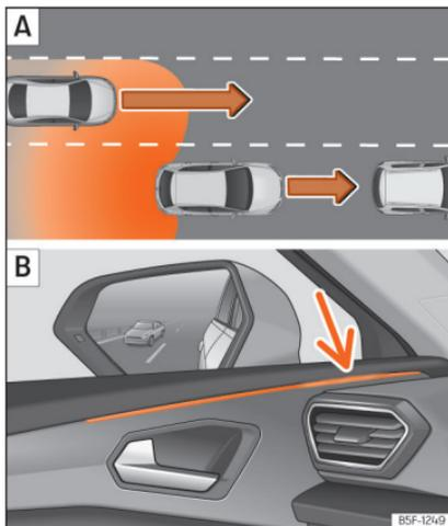
**Fig. 158** Schematic representation: **A** Passing situation with traffic behind the vehicle. **B** Indication of the lane departure warning in the control lamp on the left side.
