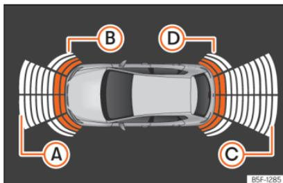
**Fig. 170** Parking Aid display on the Infotainment system screen.
