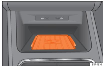
**Fig. 125** In the centre console: pad for the mobile phone connection.
