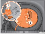
**Fig. 194** In the luggage compartment: remove the subwoofer.
