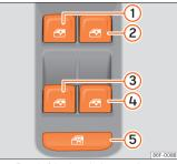
Fig. 81 Detail of the driver's door: window controls.
