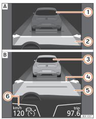
Fig. 144 On the instrument panel display: A ACC inactive (Standby). **B** ACC active.
