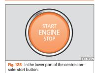
The engine can be started with a start button (Press & Drive). For this there must be a valid key inside the passenger compartment.
