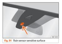
The rain sensor controls the frequency of the windscreen wiper intervals, depending on the amount of rain  $\gg \Delta$ . The sensitivity of the rain sensor can be adjusted manually. Manual wipe  $\gg$  page 114.
