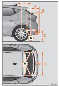
Fig. 176 Limits and attachment points for retrofitting a towing bracket.
