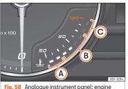
**Fig. 58** Analogue instrument panel: engine coolant temperature indicator.
