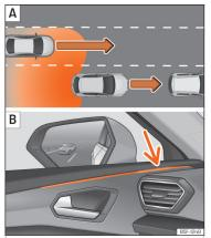
Fig. 158 Schematic representation: A Passing situation with traffic behind the vehicle. B Indication of the lane departure warning in the control lamp on the left side.
