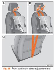
assembly according to the Top Tether belt.
