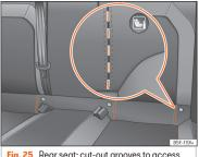
Fig. 25 Rear seat: cut-out grooves to access the ISOFIX securing rings.
