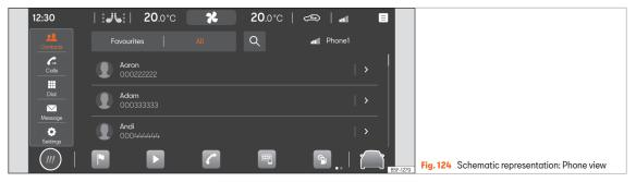
Through the telephone interface you can connect your mobile phone device suitable for telephony with the infotainment system and manage the phone functions through the infotainment system. The sound is played through the vehicle's speakers.
