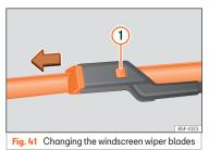
The windscreen wiper blades are supplied as standard with a layer of graphite. This layer is responsible for ensuring that the wipe is silent. If the graphite layer is damaged, the noise of the water as it is wiped across the windscreen will be louder. Check the condition of the wiper blades regularly. **If the wipers scrape across the glass**, they should be changed if they are damaged, or cleaned if they are dirty **>>> ①**.
