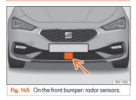
A radar sensor is fitted on the front bumper **>>> Fig. 145**.
