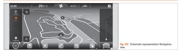
A global satellite system determines the current position of the vehicle and the sensors mounted on the vehicle analyse the routes taken. All measured values and possible traffic events are compared with the available maps to allow optimal navigation to the destination.
