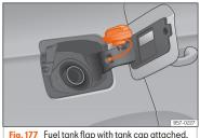
Fig. 1/7 Fuel tank flap with tank cap attached
