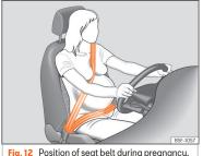
Seat belts offer their maximum protection in the event of an accident and reduce the risk of sustaining severe or fatal injuries only when they are properly positioned. Furthermore, if the webbing is correctly positioned, the seat
