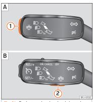
Fig. 61 On the turn signal and main beam lever: button for driver assistance systems (depending on versions).
