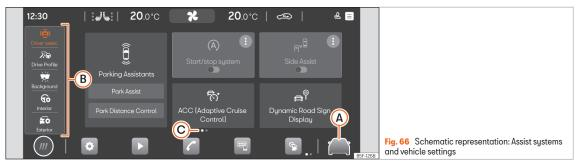
By clicking on (2) **\*\*\*** Fig. 66 (A), or in the main menu on the **Vehicle settings** symbol, the assist services menu and vehicle settings will open.
