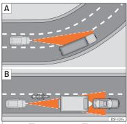
Fig. 148 A Vehicle on a bend. B Motorcyclist ahead, out of range of the radar sensor.
