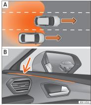
Fig. 159 Schematic representation: A Situation of an overtaking in the centre lane and then moving into the right-hand lane. B Indication of the lane departure warning in the control lamp on the right side.
