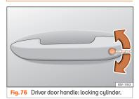
If the central locking system should fail to operate, the driver door can still be locked and unlocked by turning the key in the lock.
