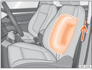
Fig. 19 Side airbag in driver's seat.
