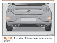
The lane departure warning uses radar sensors to monitor the areas behind the vehicle **»> Fig. 157**. The system does this by measuring the vehicle's distance from other vehicles and its speed differential. The lane departure warning will not work at speeds of less than approx. 15 km/h (9 mph).
