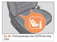
cles, the rings are secured to the seat frame and, in others, they are secured to the rear floor. The "ISOFIX" rings are located between the rear seat backrest and the seat cushioning **»** Fig. 25, **»** Fig. 26. The Top Tether rings are located on the rear part of the rear seat backrests (behind the backrest or in the luggage compartment) **>>> page 34**.
