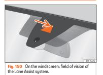
The Lane Assist System helps the driver stay in his/her lane within the physical limits of the system. This function is not suitable and is not designed to keep the vehicle automatically in the lane.
