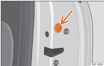
Fig. 92 Locking the door manually.
