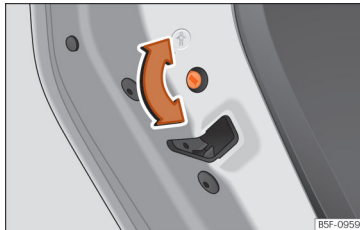
Fig. 93 Childproof lock on the left hand side door.
