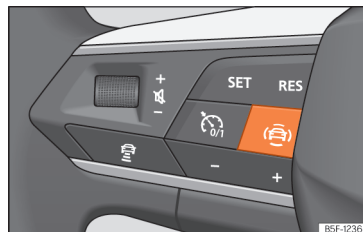
Fig. 74 Left side of the multifunction steering wheel: button for driver assistance systems (depending on versions).
