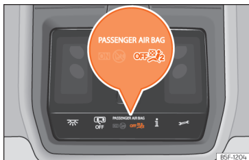
Fig. 21 On the roof console: control lamp for the deactivation of the front passenger front airbag.
