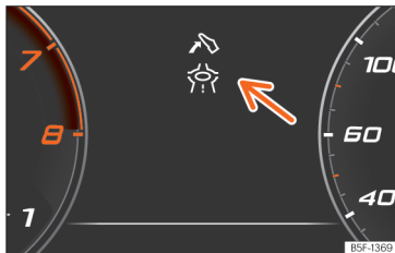
Fig. 65 Eco-efficient driving assistance indication (schematic representation).
