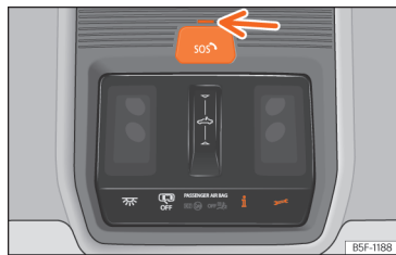
Fig. 37 On the roof console: voice service controls
