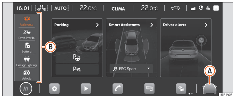
Fig. 78 Schematic representation: Assist systems and vehicle settings
