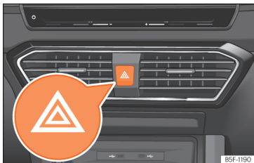
Fig. 105 Dash panel: hazard warning lights switch
