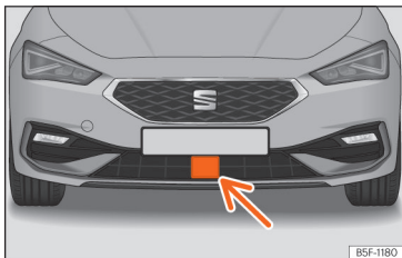
Fig. 171 On the front bumper: radar sensors.
