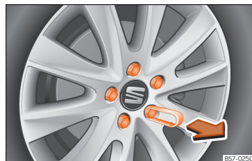
Fig. 42 Wheel: wheel nuts with caps.
