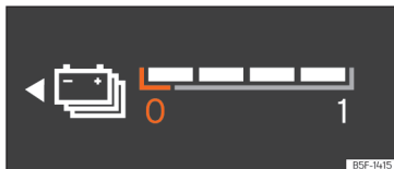
Fig. 67 Digital instrument panel: battery level indicator.
