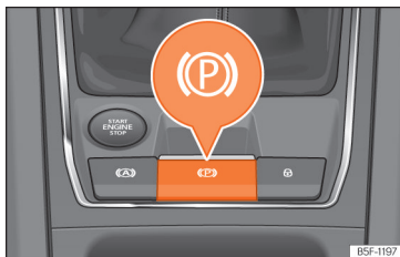
Fig. 198 In the lower part of the centre console: electronic parking brake button
