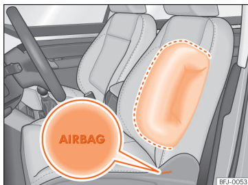
Fig. 26 Side airbag in driver's seat.
