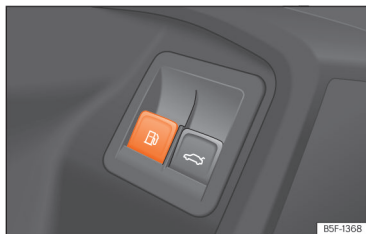
Fig. 222 Driver's door: tank flap release.
