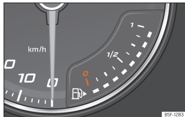
Fig. 68 Analogue instrument panel: fuel gauge
