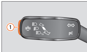
Fig. 73 On the turn signal and main beam lever: button for driver assistance systems (depending on versions).
