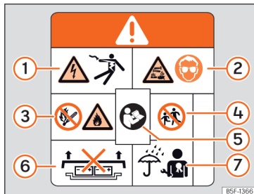
Fig. 212 High-voltage battery warning lettering.
