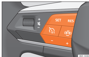
Fig. 177 On the multifunction steering wheel: buttons to operate the speed limiter.
