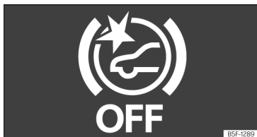
Fig. 181 On the instrument panel display: Front Assist deactivated indication.
