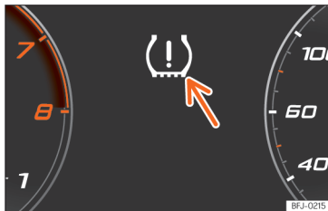
Fig. 245 Instrument panel: warning of loss of tyre pressure.
