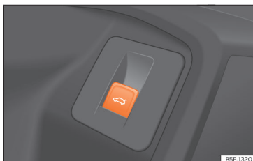
Fig. 96 On the driver's door: button to open and close the rear lid.
