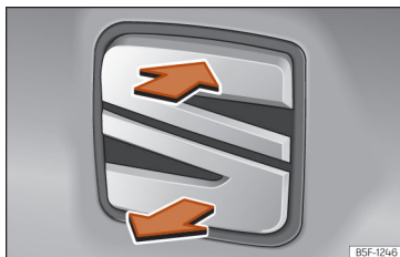
Fig. 94 Rear lid: opening from outside.
