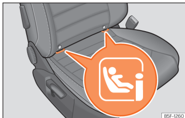
Fig. 33 Front passenger seat: ISOFIX/i-Size securing rings.
