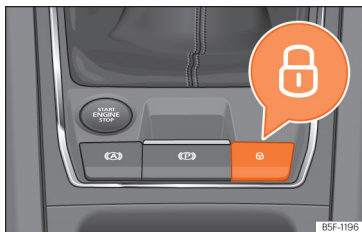
Fig. 88 In the centre console: central locking switch
