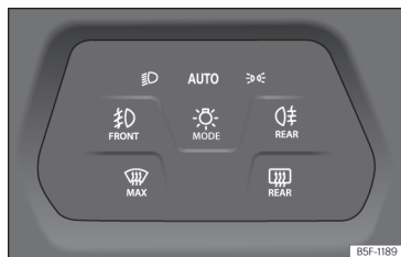
Fig. 103 Dash panel: lights control.
