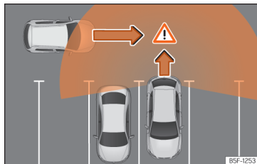
Fig. 195 Schematic representation of the rear cross traffic alert assistant: zone monitored around the vehicle while leaving a parking space.
