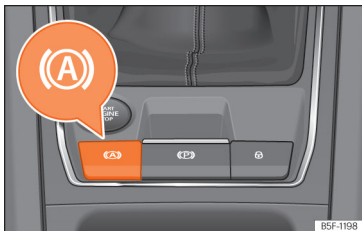
Fig. 199 In the lower part of the centre console: Auto Hold function button.
