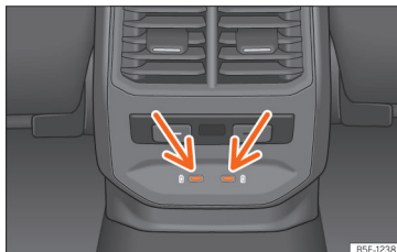
Fig. 164 Rear part of the centre console: USB connectors with power outlet function.
