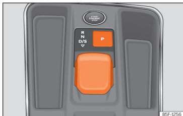
Fig. 169 In the centre console: selector lever.
