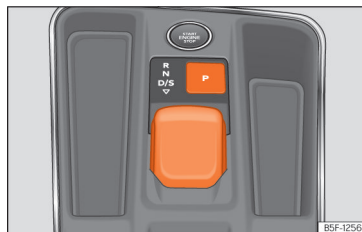
Fig. 167 In the centre console: selector lever.
