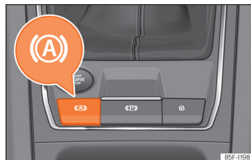
Fig. 197 In the lower part of the centre console: Auto Hold function button.
