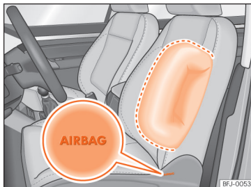
Fig. 26 Side airbag in driver's seat.
