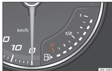
Fig. 67 Analogue instrument panel: fuel gauge
