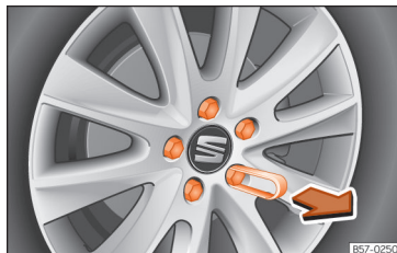
Fig. 41 Wheel: wheel nuts with caps.
