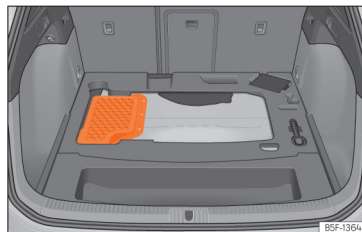
Fig. 237 Hybrid vehicles (PHEV): location of the battery in the luggage compartment
