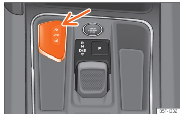
Fig. 82 Centre console: vehicle key socket.
