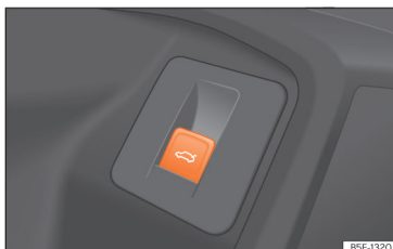
Fig. 95 On the driver's door: button to open and close the rear lid.
