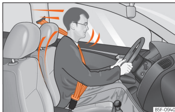
Fig. 11 Drivers with properly worn seat belts will not be thrown forward in the event of sudden braking.
