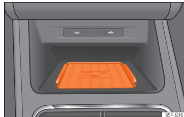
Fig. 160 In the centre console: pad for the mobile phone connection.
