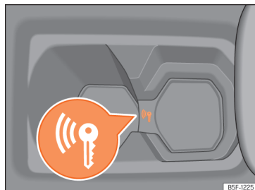
Fig. 164 In the centre console: emergency start.
