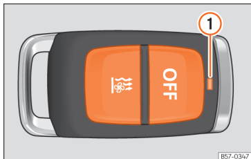
Fig. 153 Auxiliary heating: radio-operated remote control.
