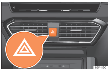
Fig. 104 Dash panel: hazard warning lights switch
