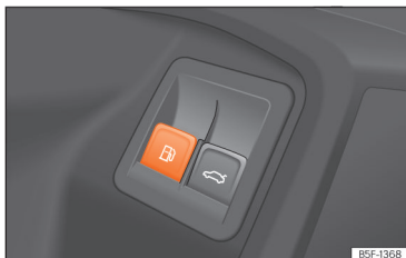
Fig. 220 Driver's door: tank flap release.
