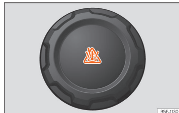
Fig. 234 Engine compartment: coolant expansion tank cap.
