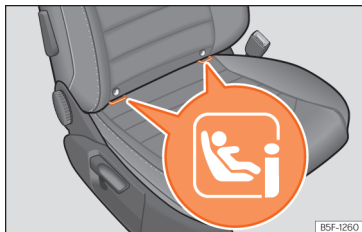
Fig. 33 Front passenger seat: ISOFIX/i-Size securing rings.
