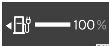
Fig. 66 Digital instrument panel: battery level indicator.
