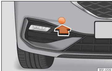
Fig. 51 On the right side of the front bumper: remove the cover.
