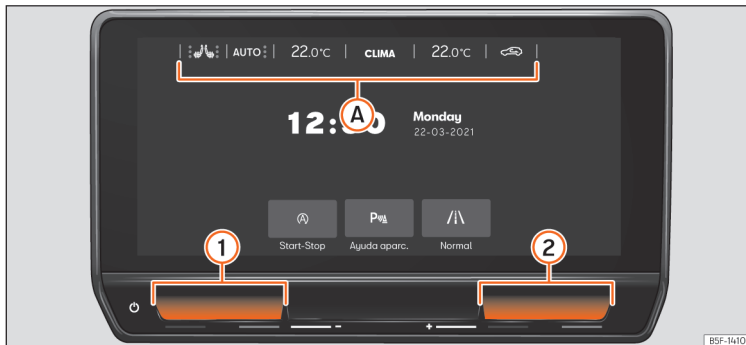
Fig. 111 Schematic representation: air-conditioning functions.
