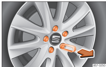
Fig. 239 Wheel: wheel bolts with caps.
