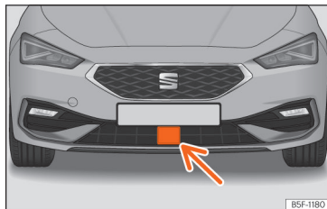
Fig. 123 On the front bumper: radar sensor.
