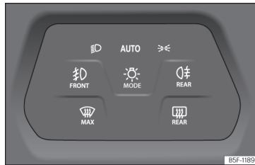
Fig. 101 Instrument panel: light panel.
