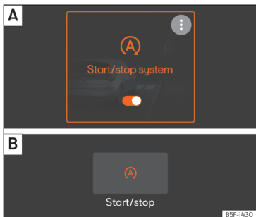
Fig. 117 On the infotainment system display: Start-Stop system on. A View in the main menu. B View with the Infotainment system off.
