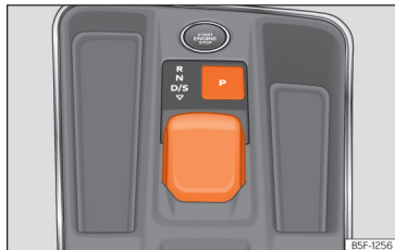
Fig. 119 On the centre console: selector lever.
