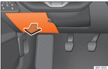
Fig. 216 On the dashboard on the driver side: lid of the fuse box.
