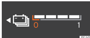
Fig. 9 Digital instrument cluster: battery level indicator.
