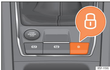
Fig. 74 On the centre console: central locking switch
