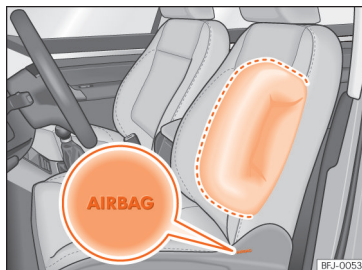
Fig. 36 Side airbag in driver's seat.
