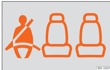
Fig. 23 Instrument cluster: indication of the status of the rear seat seat belts.
