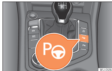
Fig. 279 In the centre console, top section: button to switch on the Park Assist system.
