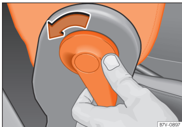
Fig. 149 Unlocking the folding backrest of the front passenger seat
