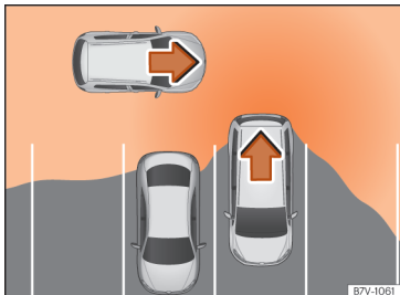
Fig. 277 Diagram of the parking assistant: detected area around the vehicle that is driving off.
