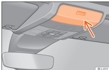
Fig. 174 On the roof console: compartment for glasses.
