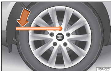
Fig. 75 Wheel: loosen the wheel bolts.
