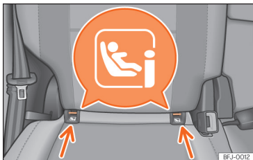
Fig. 37 Side seats on the second row: ISOFIX/i-Size fastening rings.
