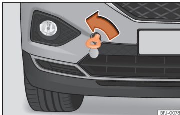
Fig. 79 Right side of the front bumper: towline anchorage screwed in.
