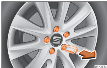
Fig. 73 Wheel: wheel bolts with caps.
