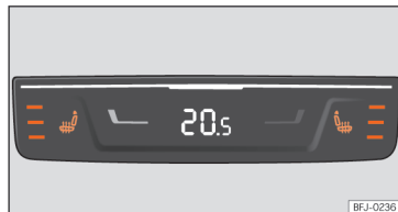
Fig. 14.9 In the rear part of the centre console: rear seats heating switch.
