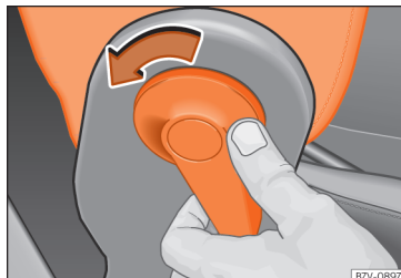
Fig. 114 Unlocking the folding backrest of the front passenger seat
