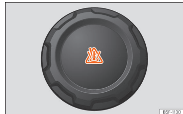
Fig. 246 Engine compartment: coolant expansion tank cap.
