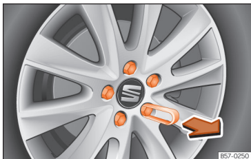
Fig. 33 Wheel: wheel nuts with caps.
