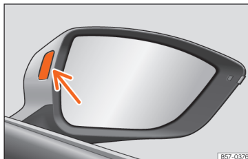
Fig. 194 Control lamp of the lane departure indicator lamp in external rear view mirrors.
