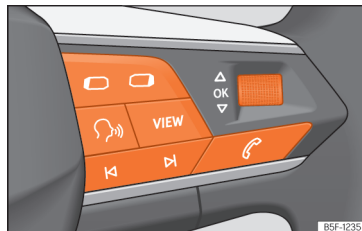
Fig. 63 Right side of the multifunction steering wheel: buttons to the menus and information displays on the instrument panel.
