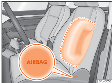
Fig. 21 Side airbag in driver's seat.
