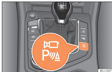
Fig. 214 Centre console: button to manually activate/deactivate the peripheral vision system when combined with the park assist system.
