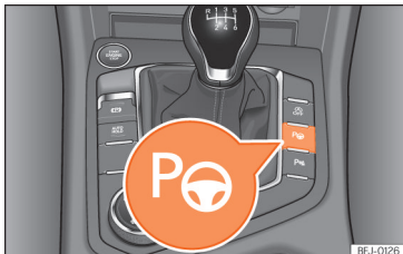
Fig. 200 In the upper part of the centre console: button to switch on the Park Assist system.
