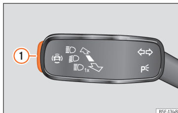
Fig. 64 On the turn signal and main beam lever: button for driver assistance systems (depending on versions).
