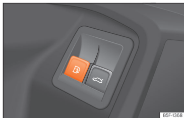
Fig. 233 Driver's door: tank flap release.
