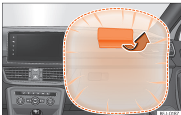
Fig. 16 Front passenger airbag located in dash panel.
