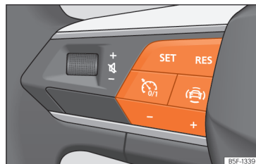
Fig. 180 On the multifunction steering wheel: buttons to operate the speed limiter.
