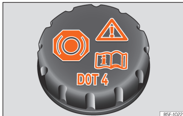
Fig. 247 Engine compartment: brake fluid reservoir cap.
