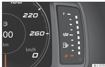
Fig. 61 Digital instrument panel: fuel gauge.
