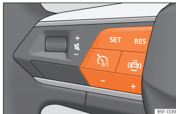
Fig. 182 On the multifunction steering wheel: buttons to operate the speed limiter.
