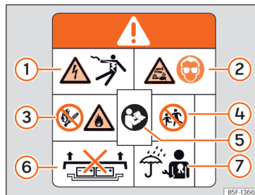
Fig. 224 High-voltage battery warning lettering.
