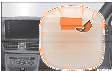
Fig. 16 Front passenger airbag located in dash panel.
