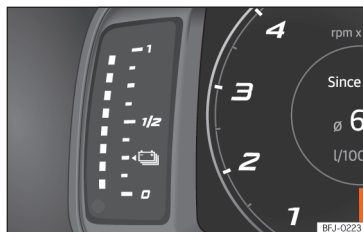
Fig. 60 Instrument panel: battery level indicator.
