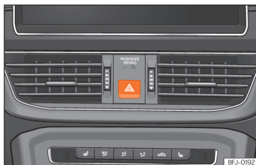
Fig. 96 Dash panel: hazard warning lights switch
