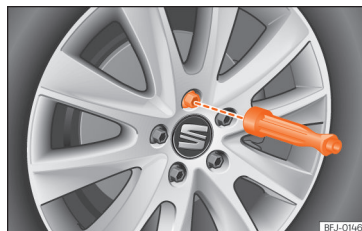
Fig. 39 Wheel change: loosen wheel nuts with the socket in the handle of the screwdriver.
