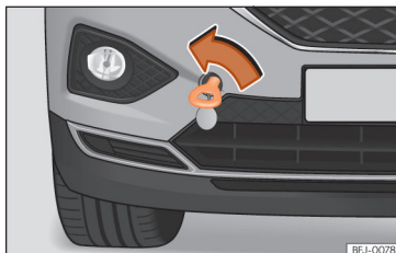
Fig. 46 On the right side of the front bumper: towline anchorage in position.
