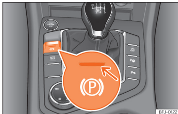
Fig. 200 In the lower part of the centre console: electronic parking brake button
