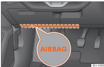
Fig. 19 On the driver side: location of the knee airbag
