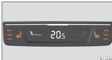
Fig. 151 In the rear part of the centre console: rear seats heating switch.
