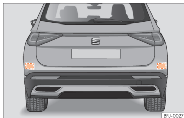
Fig. 178 Rear view of the vehicle: radar sensor zones.
