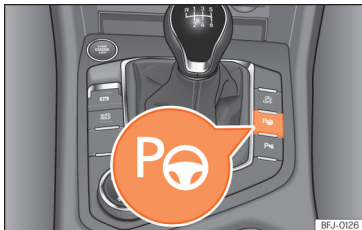
Fig. 202 In the upper part of the centre console: button to switch on the Park Assist system.
