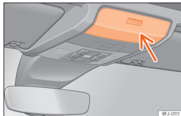
Fig. 139 On the roof console: glasses case.
