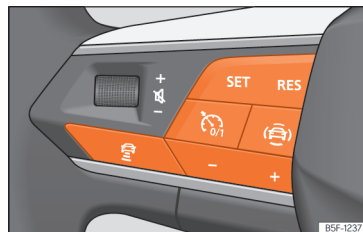
Fig. 186 On the multifunction steering wheel: buttons to operate the ACC
