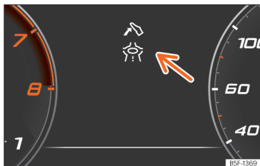
Fig. 58 Eco-efficient driving assistance indication (schematic representation).
