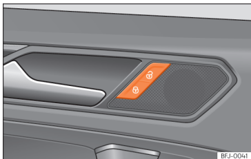
Fig. 77 Driver's door: central locking switch.
