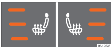
Fig. 150 In the centre console: front seat heating switches.
