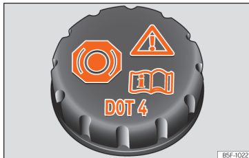
Fig. 249 Engine compartment: brake fluid reservoir cap.
