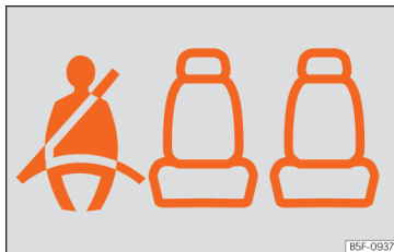
Fig. 6 Instrument panel: left rear seat occupied and corresponding seat belt fastened display.
