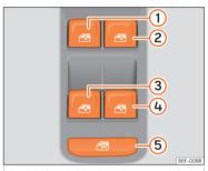
**Fig. 80** Detail of the driver door: controls for the windows.
