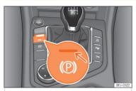
**Fig. 154** Centre console, lower part: electronic parking brake button.
