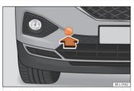
Fig. 224 Front bumper on right: remove the lid.
