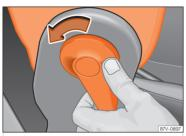
**Fig. 90** Unlocking the folding backrest of the front passenger seat
