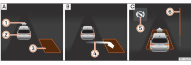
Fig. 164 On the instrument cluster displau: parallel parking. A: Finding a parking space B: Parking position, C: Manoeuvring.
