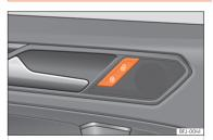
**Fig. 70** On the driver's door: central locking button.
