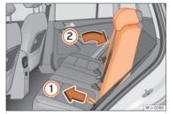
Fig. 92 Rear seat backrest adjustment.
