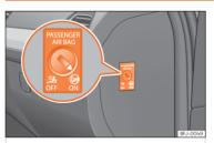
**Fig. 32** Switch for activating and deactivating the front passenger airbag.
