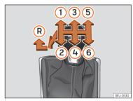
Fig. 122 Diagram of a 6-speed manual gearbox.
