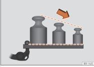
**Fig. 211** Recommended weight distribution on the rear support sustem.
