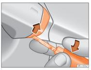
**Fig. 72** Driver's door handle: pry the cover open.
