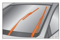
Fig. 219 Wipers in service position.
