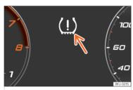
**Fig. 257** Instrument panel: warning of loss of tyre pressure.
