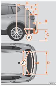
**Fig. 213** Limits and attachment points for retrofitting a towing bracket.
