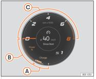
Fig. 11 Digital instrument cluster: Power meter
