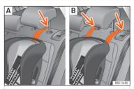
**Fig. 44** Rear seats: adjustment and assembly according to the Top Tether belt.
