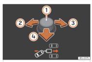
**Fig. 172** Outside rearview mirror rotary control: adjust the trailer angle.
