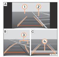
**Fig. 167** Display on the infotainment system screen; parking with the reverse assistant.
