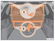
Fig. 203 Net partition fitted.
