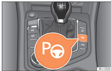
Fig. 161 In the centre console: button to switch on the Park Assist system.
