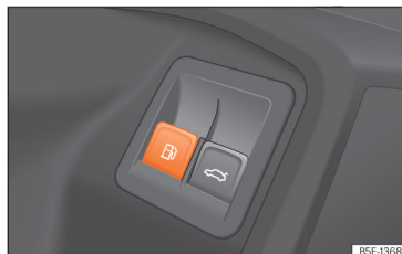
Fig. 215 Driver's door: tank cover release.
