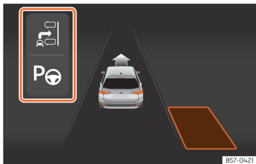
Fig. 162 On the instrument panel display: display of the assisted parking system with decreased visibility.
