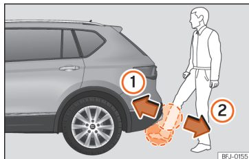
Fig. 78 Rear lid with sensor-controlled opening (Easy Open).
