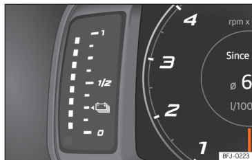
Fig. 8 Instrument cluster: battery level indicator.
