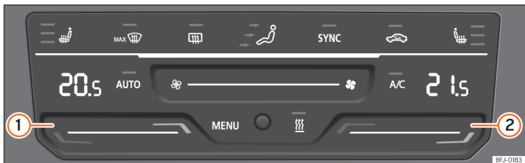
Fig. 112 In the centre console: Climatronic control panel.
