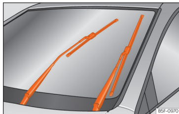
Fig. 219 Wipers in service position.
