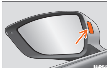
Fig. 150 Control lamp of the lane departure warning.
