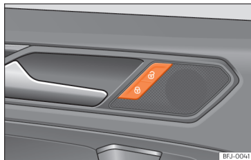
Fig. 70 On the driver's door: central locking button.
