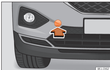
Fig. 224 Front bumper on right: remove the lid.
