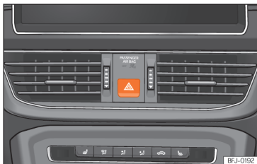
Fig. 49 Dashboard: switch for hazard warning lights.
