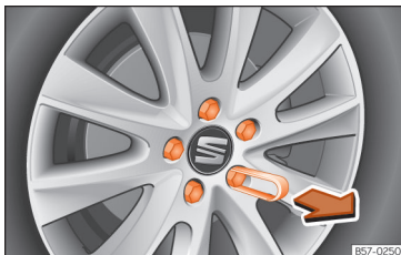
Fig. 250 Wheel: wheel bolts with caps.
