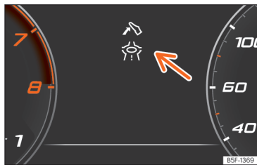
Fig. 14 Eco-efficient driving assistance indication (schematic representation).
