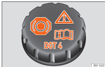
Fig. 237 Engine compartment: brake fluid reservoir cap.
