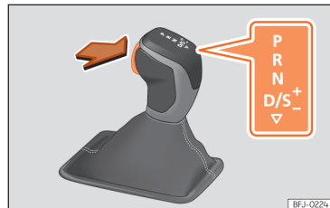
Fig. 123 Selector lever lock.
