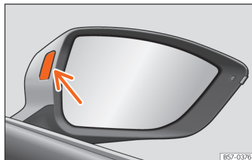
Fig. 151 Control lamp of the lane departure warning.
