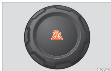
Fig. 236 Front compartment: coolant expansion tank cap.
