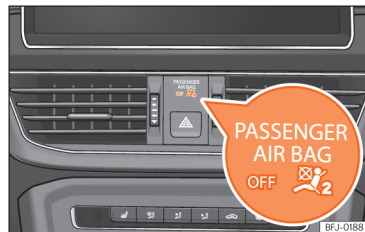
Fig. 33 Dashboard: control lamp for deactivated front passenger airbag in centre console.
