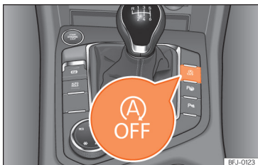
Fig. 121 Centre console: Start-Stop system button.
