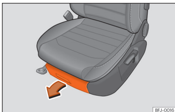
Fig. 181 Storage compartment under the right front passenger seat.
