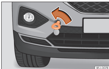
Fig. 225 Right side of the front bumper: towline anchorage screwed in.
