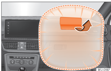
Fig. 31 Front passenger airbag located in dash panel.
