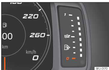
Fig. 7 SEAT Digital Cockpit instrument cluster: fuel gauge.
