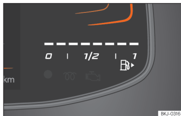
Fig. 6 Basic instrument cluster: fuel gauge.
