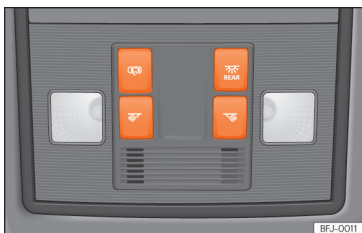
Fig. 106 Detail of headliner: front interior lighting.
