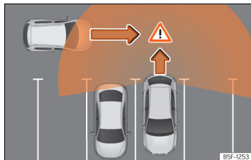
Fig. 174 Diagram of the parking assistant: detected area around the vehicle that is driving off.
