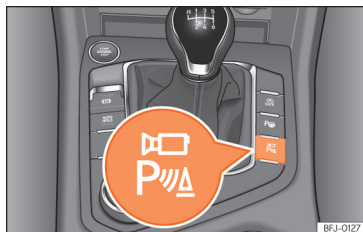
Fig. 170 Centre console: button to manually switch on/off the Top View camera system when in combination with the parking assist system.
