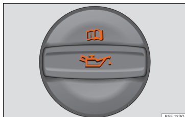
Fig. 242 Oil filler cap cover in the engine compartment.
