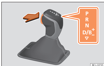
Fig. 124 Selector lever lock (hybrid vehicles).
